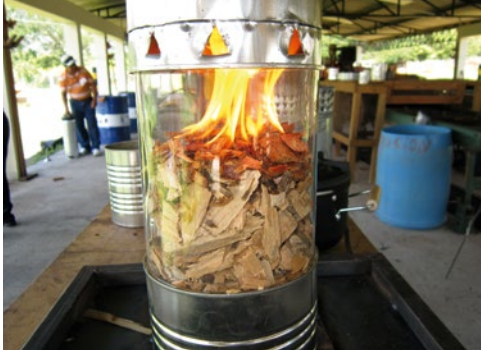
Photo 2.2 A stack of woodchips in a fuel container made of heat-resistant glass lit on top, directly after lighting
