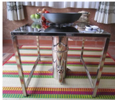
Photo 4.64 The 150 gasifier in a stainless-steel enclosure
