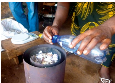
Photo 2.17 Metering kerosene with a bottle top before sprinkling it onto the fuel
