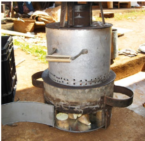
Photo 2.10 Roasting potatoes in the baking tray underneath the charcoal
