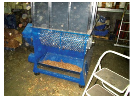
Photo 3.13 Ground material exiting through the 12 mm screen
