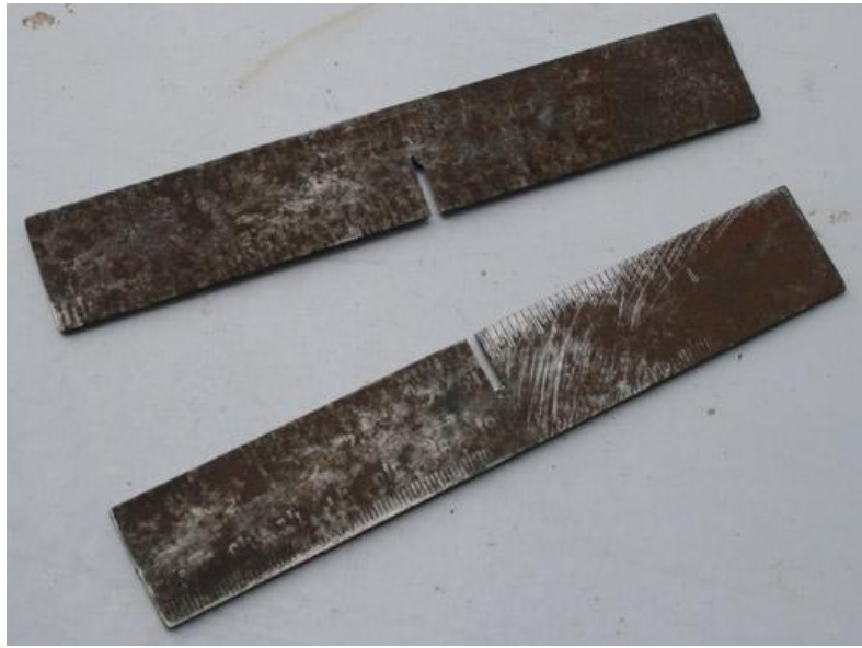
Figure 17: 3 Flat steel with grooves cut
