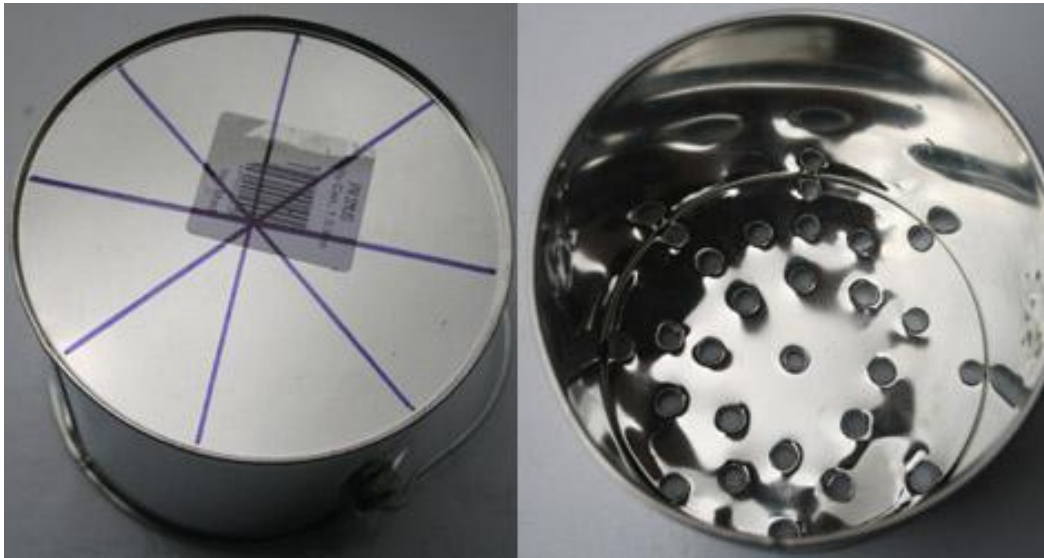
Figure 10: Primary air holes in Fuel Chamber (Billy C).
