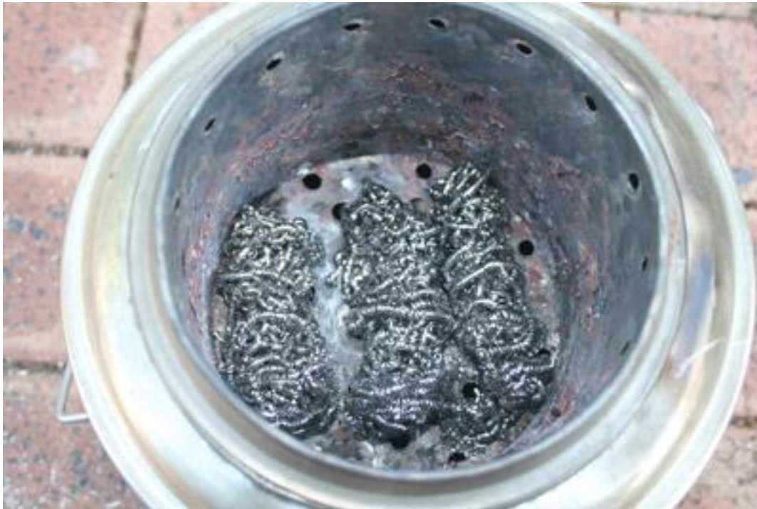
Figure 21: Stainless steel pot scrubbers in base of fuel chamber
