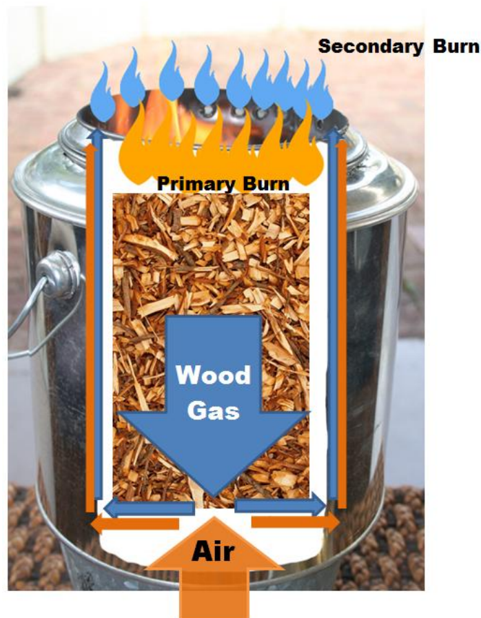
Figure 2: TLUD principle
