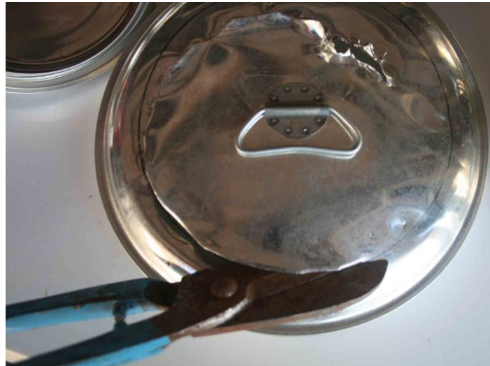
Figure 8: Cutting the centre of Billy Lid A
