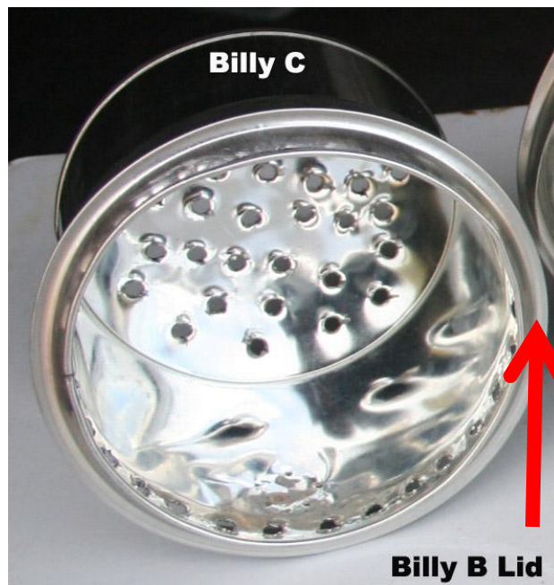
Figure 13: Fuel Chamber (Billy C) inserted into Billy B Lid.
