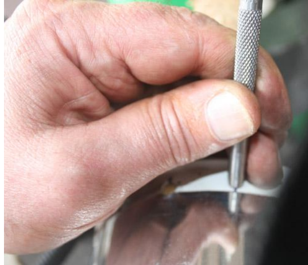
Figure 12: Punching secondary burn holes in Fuel Chamber (Billy C).
