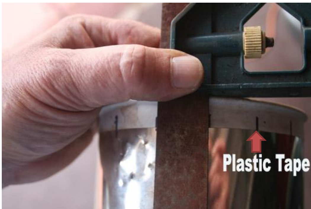
Figure 11: Marking secondary burn holes in Fuel Chamber (Billy C).
