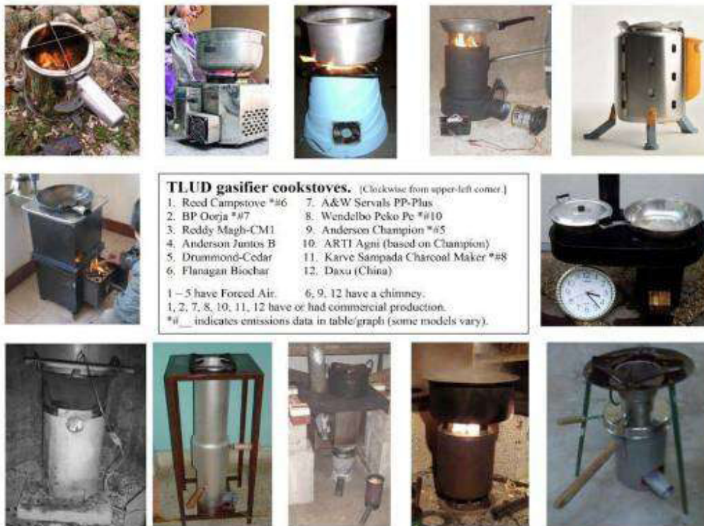
Figure 4: A range of top-lit updraft (TLUD) stoves, source [11]
