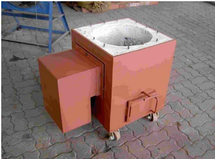
Figure 18: Primary Air Inlet attached to the Reaction Chamber
