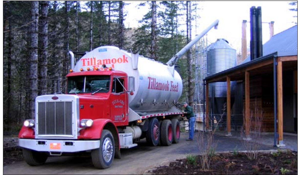
Using a grain auger from the delivery truck, the silo is refilled about 2-3 times per year. Photo: Oregon Dept. of Forestry.
