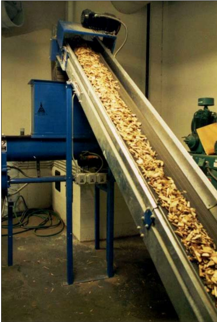
This fully automated inclined chip conveyer moves chips from the storage bin to the combustion chamber. Photo: BERC.
