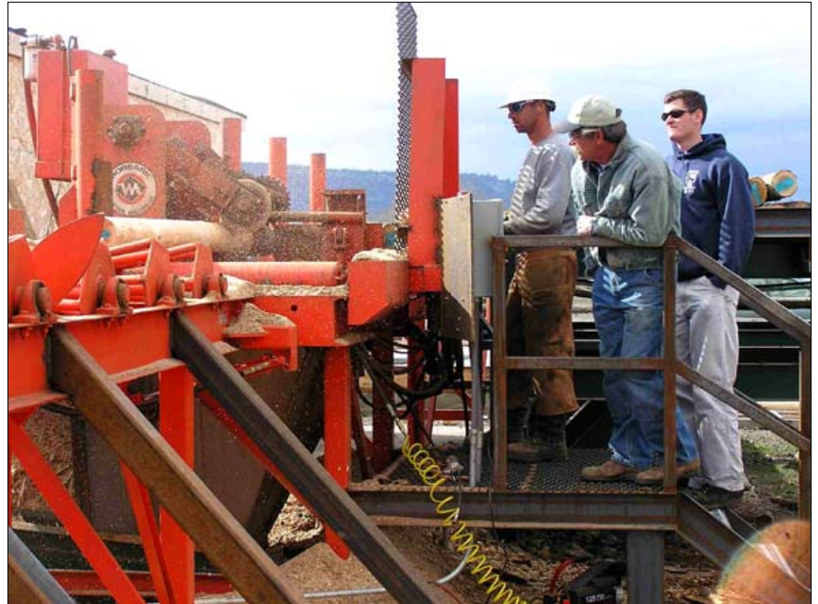
Log peeling at Community Smallwood Solutions. Photo: Wallowa Resources
