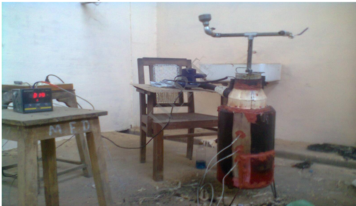
Figure 3.1 Experimental setup of updraft biomass gasifier
