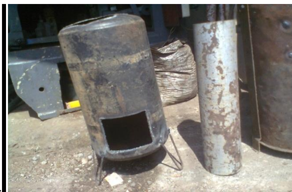
Figure 2.3 Cutting of the air tank
