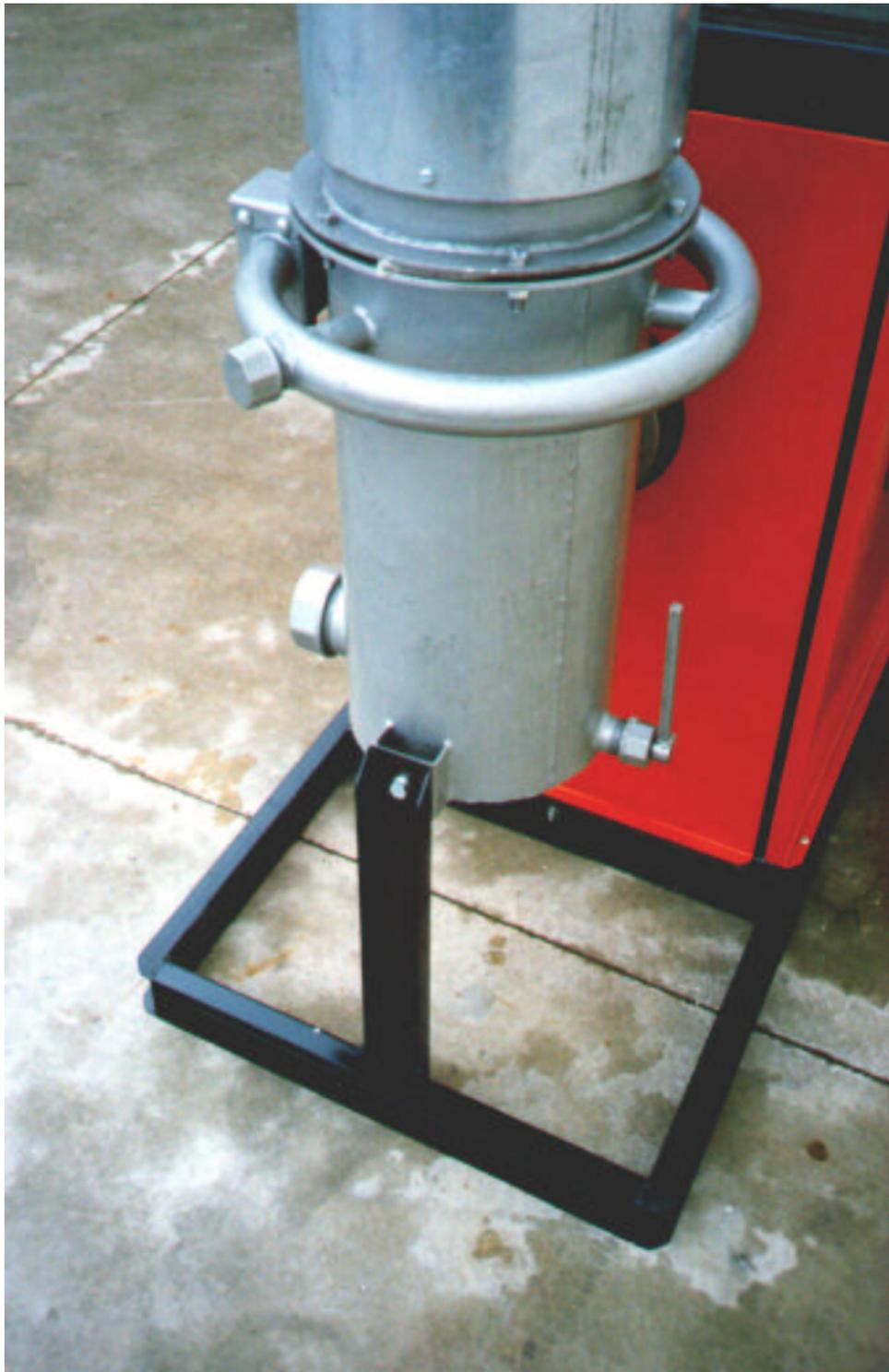
This was the original size of the Pioneer Class hearth and fuel hopper, but the narrow hopper caused fuel flow problems. We fitted a larger hopper, hence the taper on the drawing above the nozzles. It is easier to just have the larger parallel cylinders.
