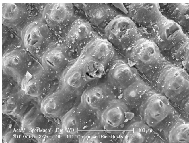
Fig. 2. Scanning Electron Micrograph (SEM) of rice husk char, showing the intact structure of the external silica shell.
