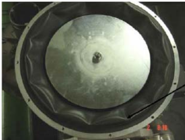
Figure 7-4: Swollen synthetic membrane in the gas control system of the Spiez plant [55]
