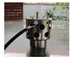
A state-of-the-art electronic speed regulator is tucked away within the fan housing right above the fan. With an easy turn of a dial, the operator can control the flow of gas. This DC fan on loose rice hulls consumes no more than a watt or two of electricity.
