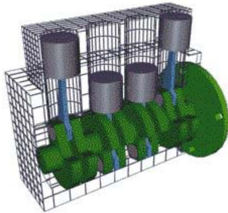
Pistons moving up and down inside the cylinders
