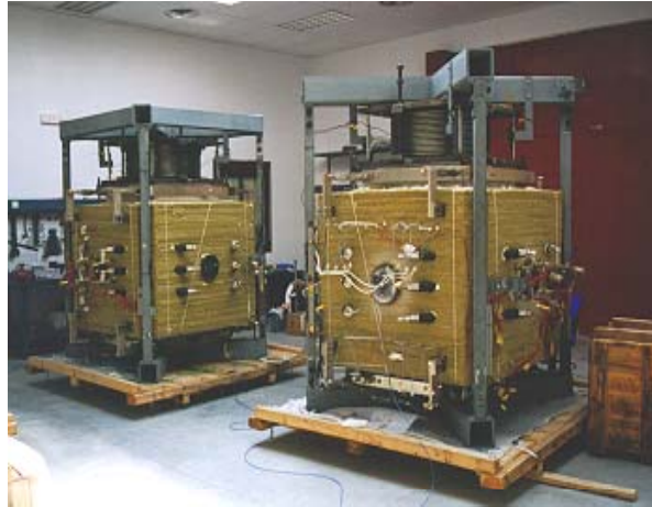
100 kW modules for MCFC plants (Ansaldo Ricerche laboratories)
