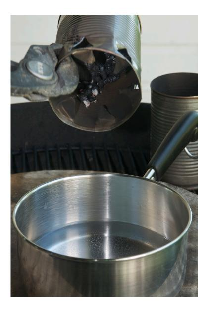
Wearing insulated gloves, use the pliers to slowly pour the very hot biochar into the 250 ml of cold water in the quenching pot. Make sure ALL of the hot pieces of biochar get into the pot and that none are left in the TLUD. You may have to tap the bottom of the TLUD quite hard to jar any stuck bits free. Do a careful visual check of the TLUD to make sure it is completely empty.
