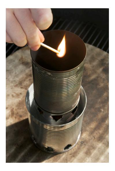
Simply drop the match down the draft can and into the basic TLUD can below. The alcohol soaked starter pellets will light immediately. Start your timer NOW so you can time the run.
