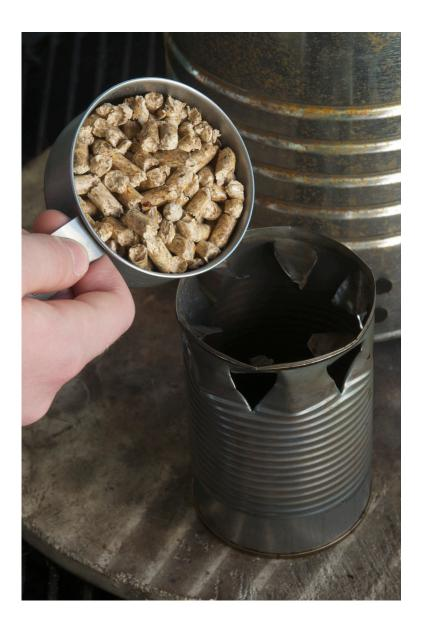
The main part of the TLUD is the can with the primary and secondary air holes in it.
