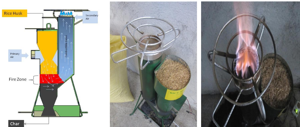
Figure 2. Schematic Drawing and Pictorials of the Operation of the Stove.
