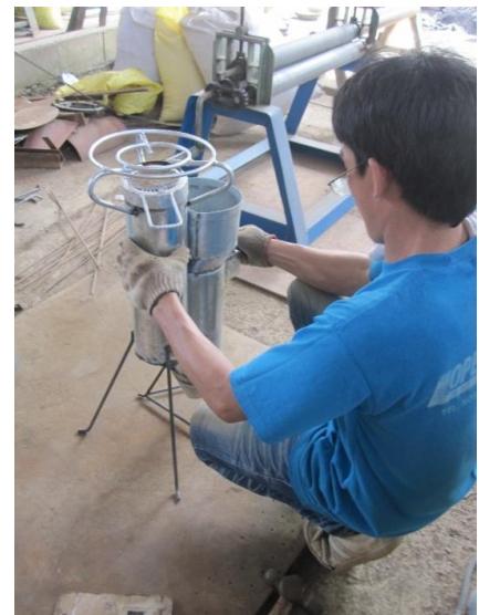
Figure 3. Fabrication of the Stove in a Small Backyard Shop.
