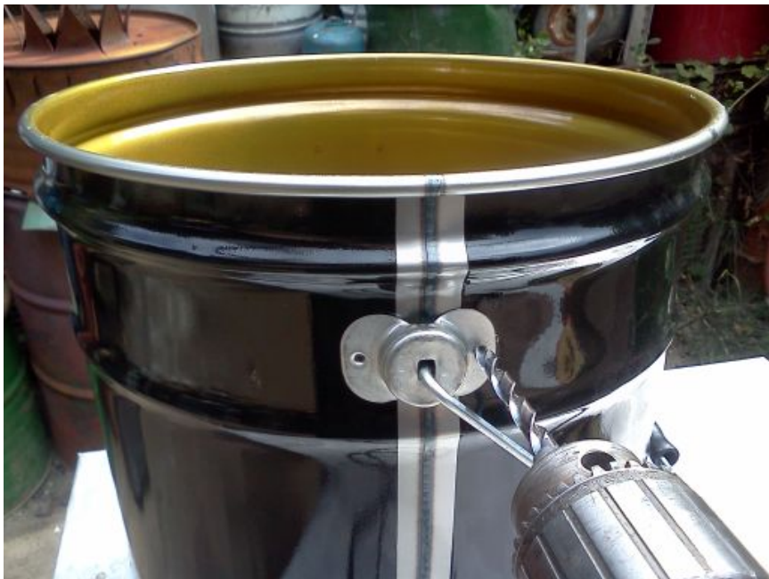
Handle Spot Weld Removal
