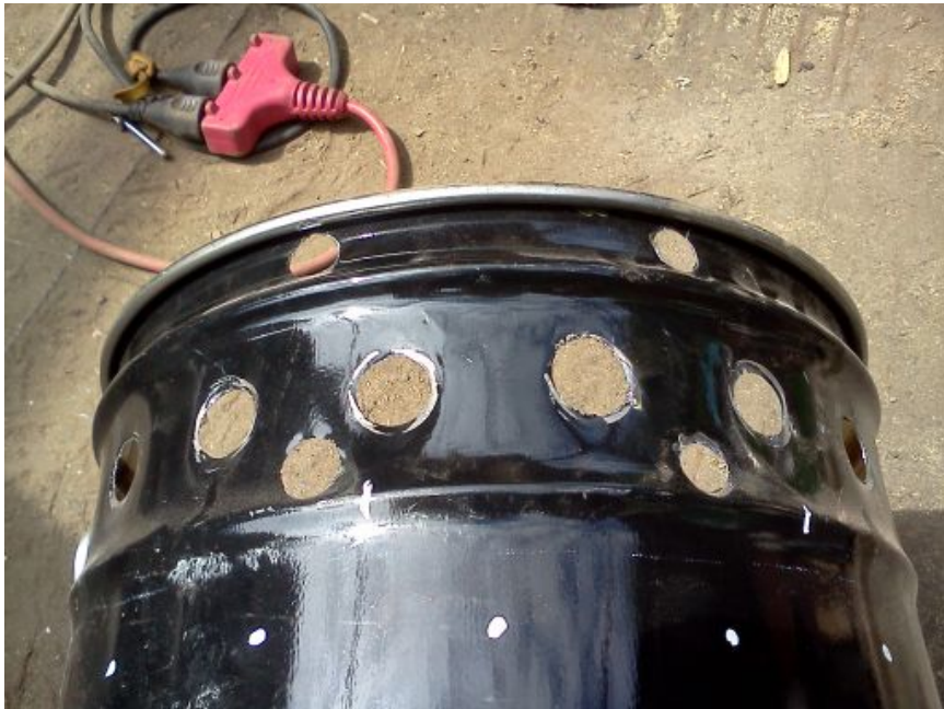
CookTop Pattern Closeup - rebar holes to be 3/8in
