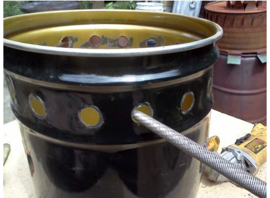
Inside Edges Still Sharp - Use Round Rasp
