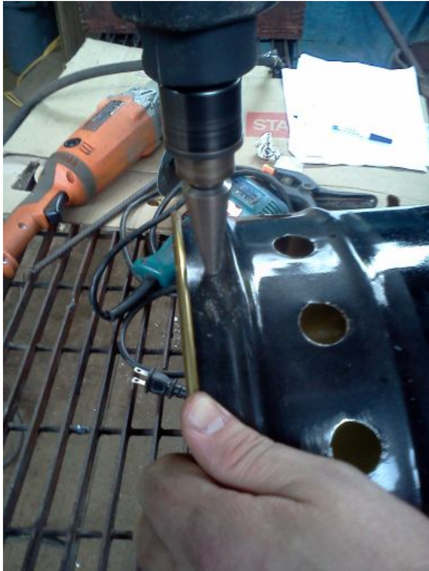
Finish up with Step Drill (make hole only as big as needed)
