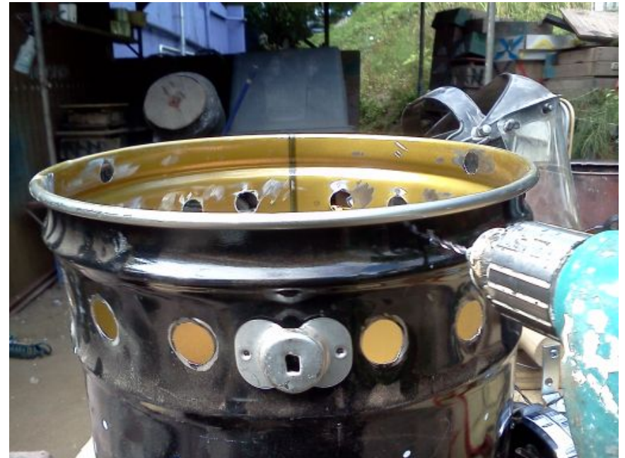
Drilling Cook Top handle holes
