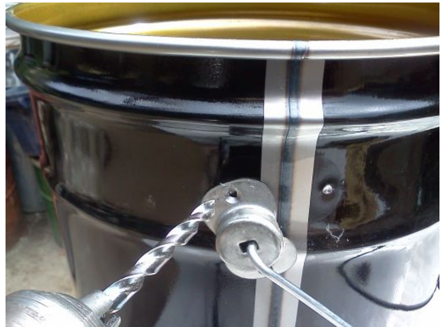
Second Spot Weld Removal
