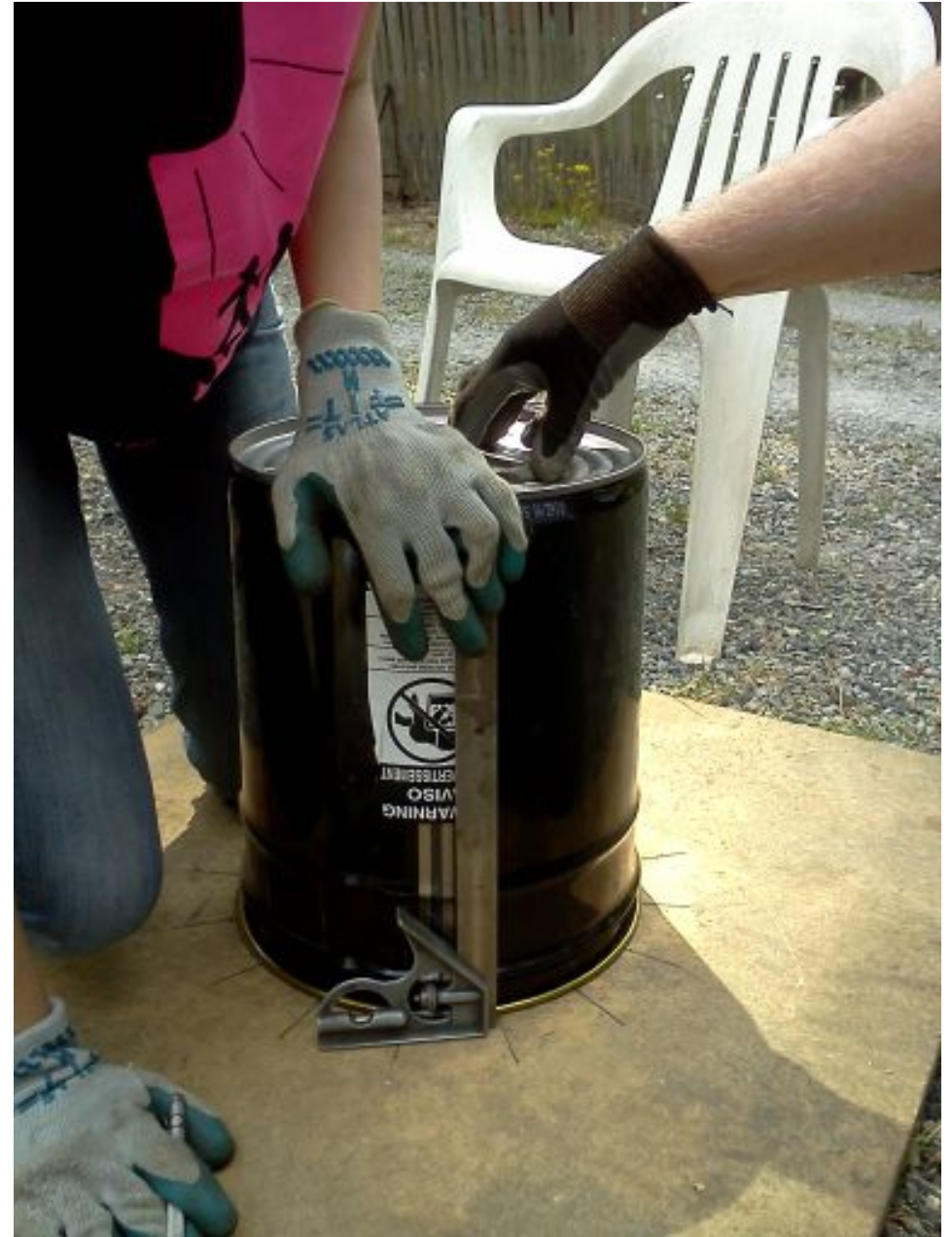
Use Right Angle to Scribe hole pattern This is also a good time to remove any labeling on the outside of the bucket
