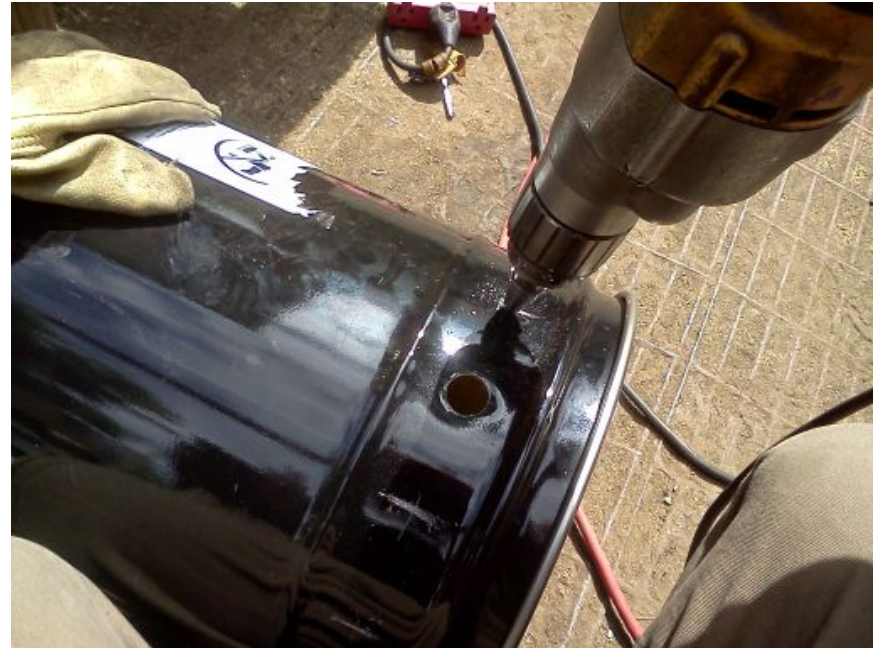
Drilling Stove Secondary Air Holes
