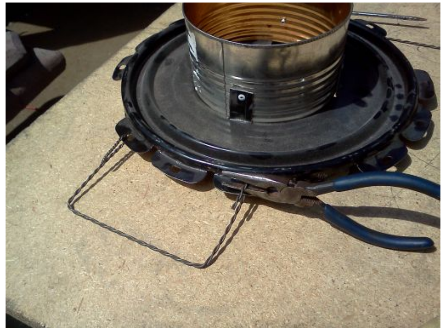
Bend Both Sides to Wrap w Thinner wire
