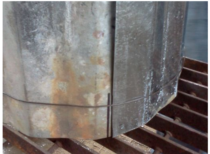
Use Wires to hold - better yet use Vice Grips
