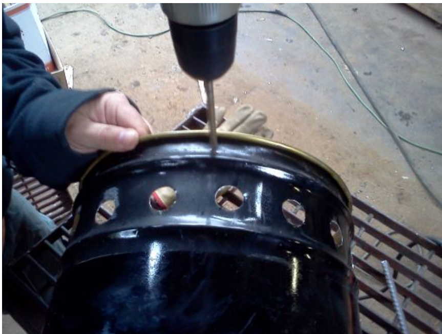
Drill centered re-bar pilot hole - use smaller bit
