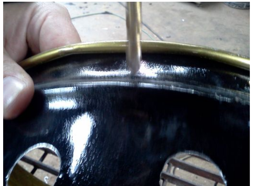
Should be centered between top and ridge
