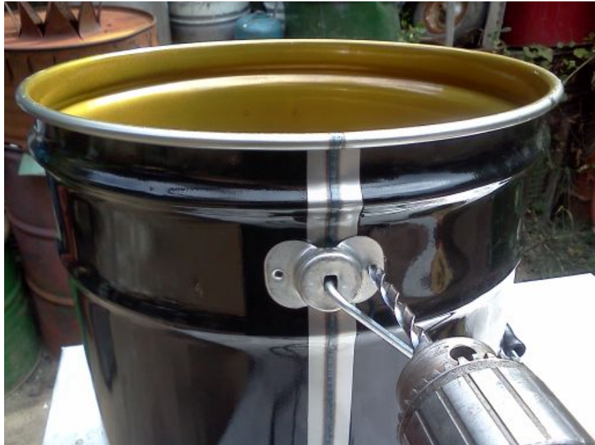
Handle Spot Weld Removal
