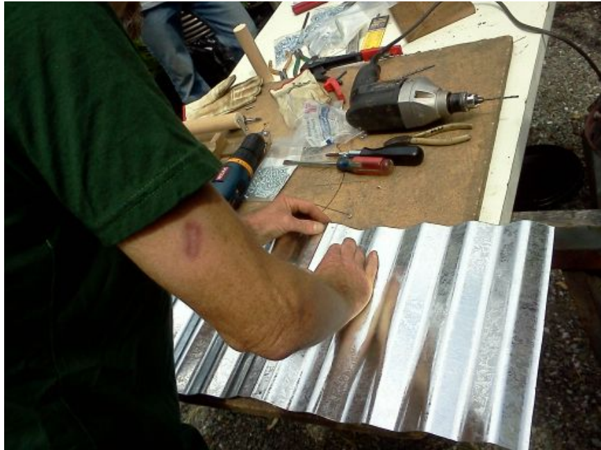
Align large and small shroud pieces
