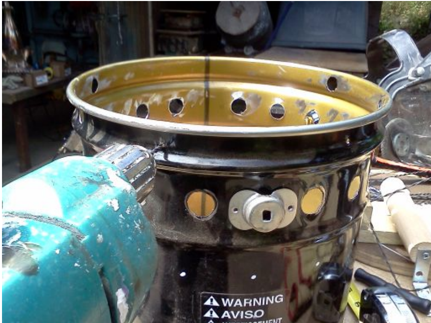
Drilling 2nd Cook Top Handle Holes
