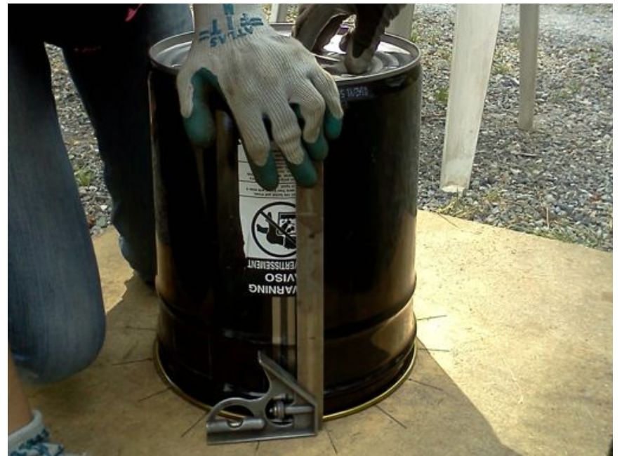
Use Right Angle to Scribe hole pattern
