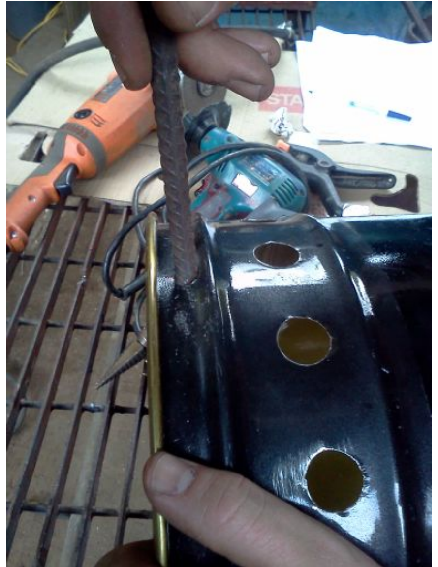
Measure for size (too big a hole is no good)
