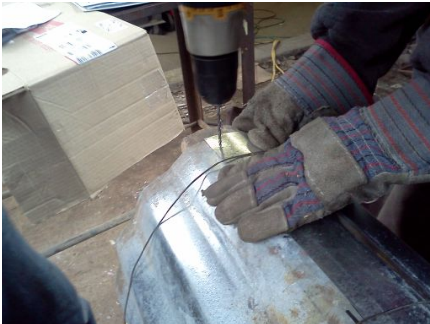
Align & Drill other Shroud End
