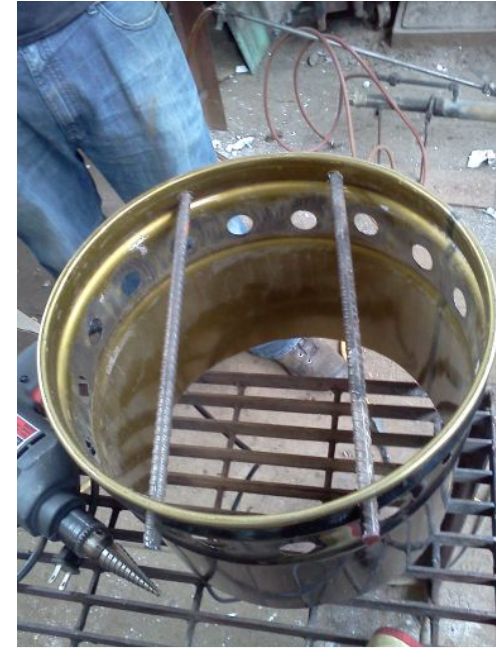
Re-bar holes sized, centered, and installed
