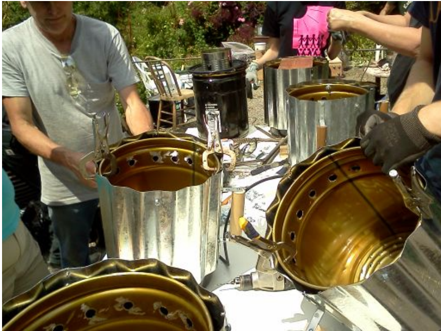
Clamp Shroud to Stove body then Drill
