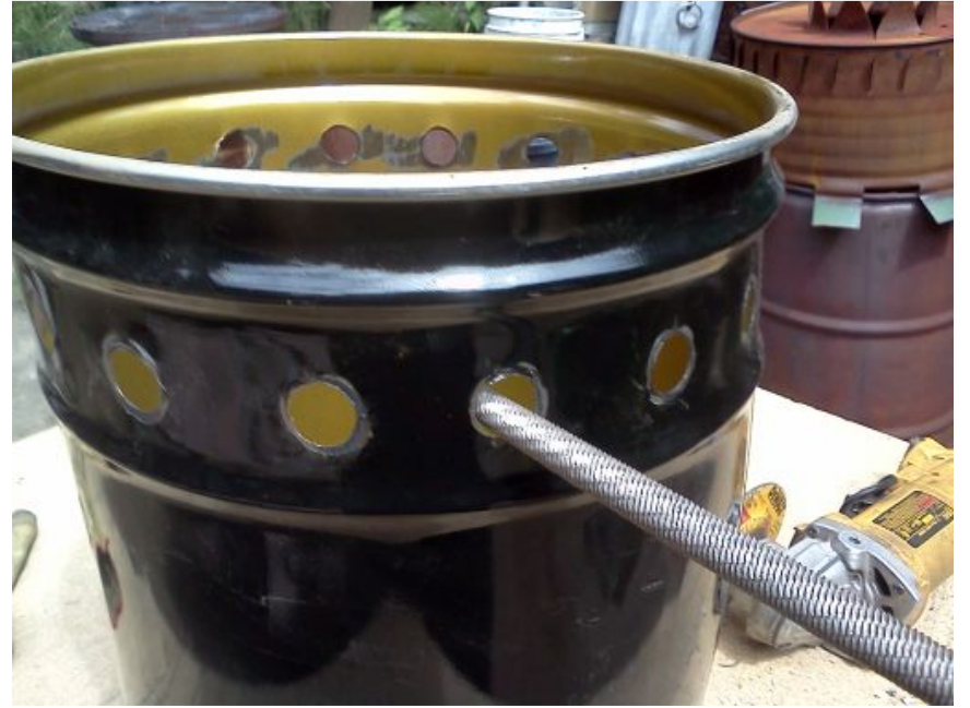
Inside Edges Still Sharp - Use Round Rasp
