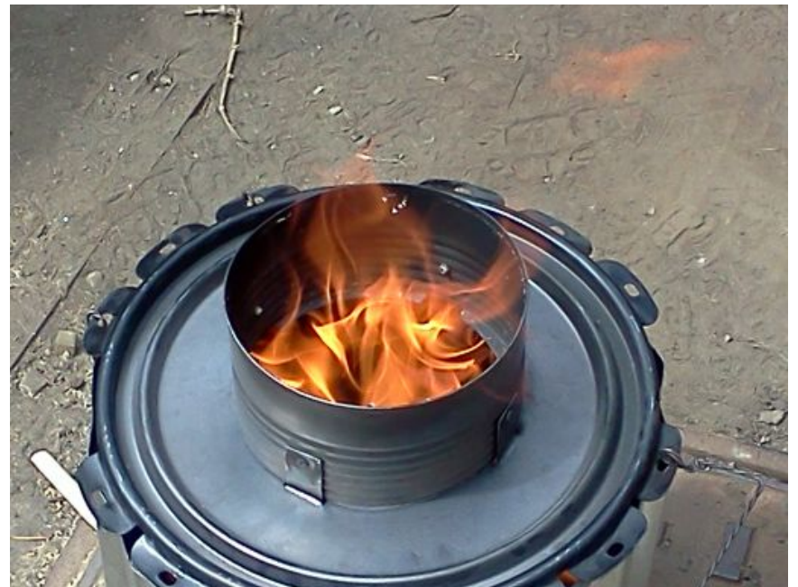
Keep up Wind - Smells Until Burns Paint Off
