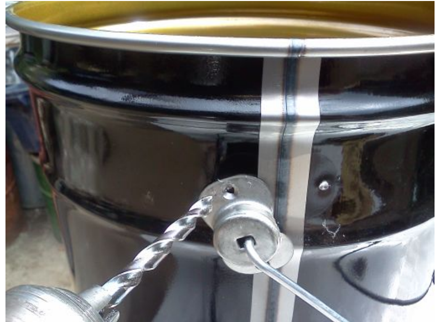
Second Spot Weld Removal
