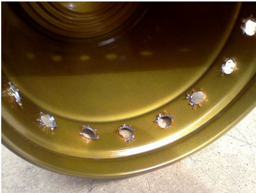
Sharp Burrs on Back of Holes
