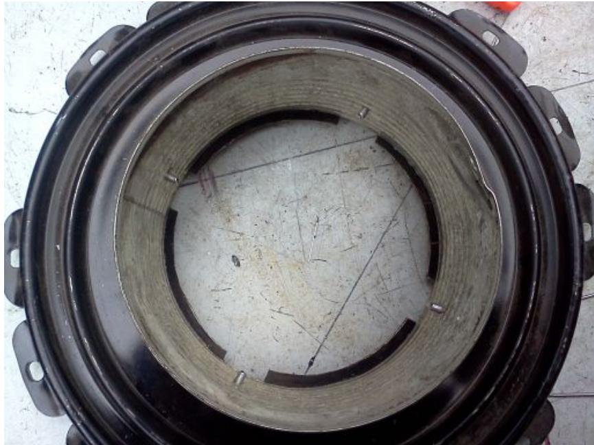
Lid Rivets Complete - inside view
