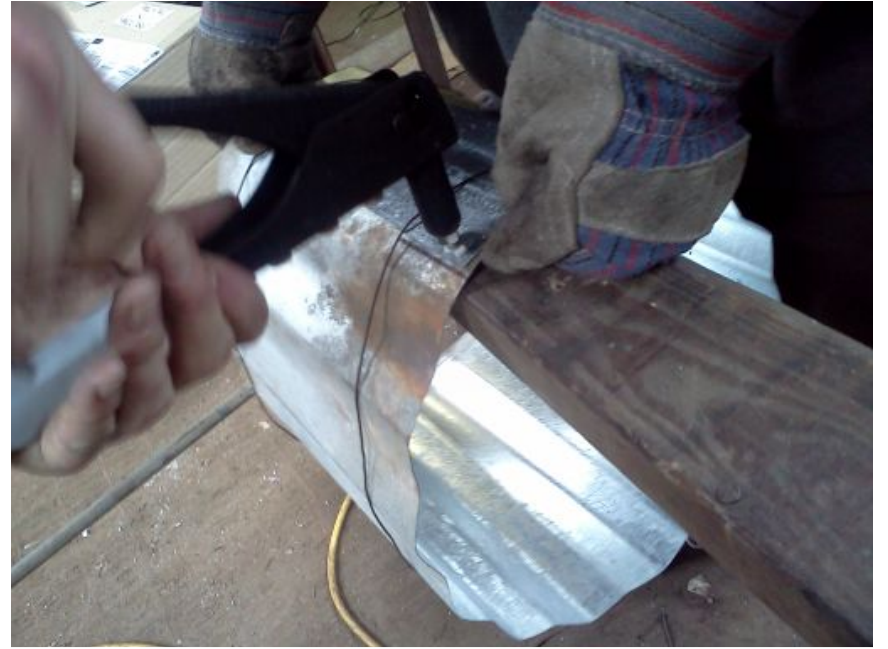
Rivet Shroud End
