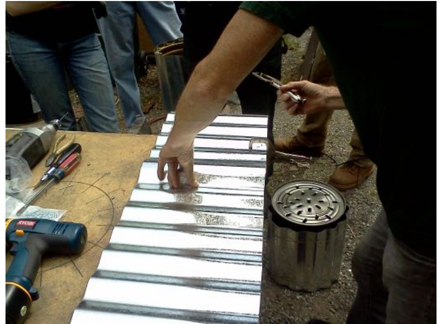
Vice Grip together, Drill, and Rivet
