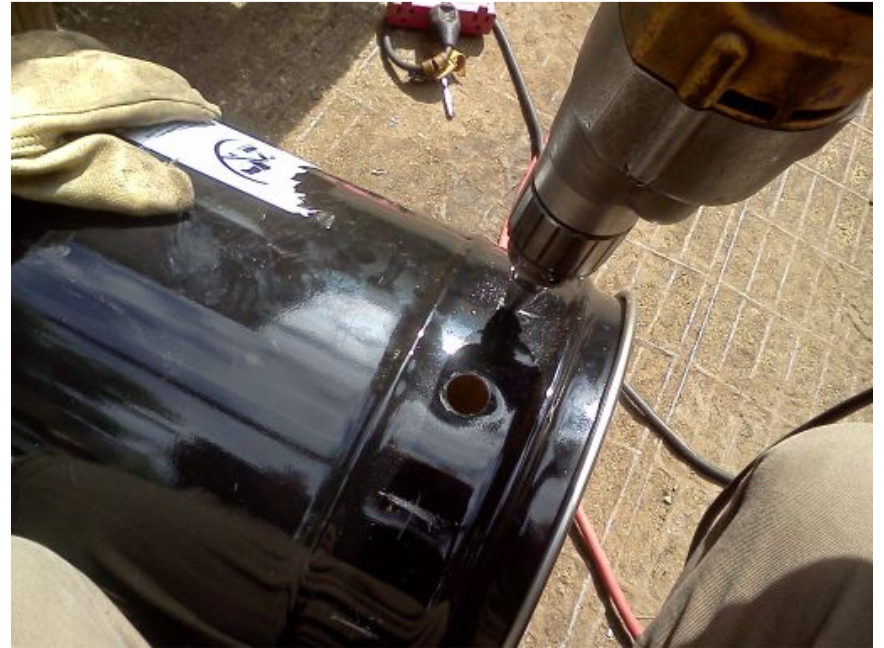
Drilling Stove Secondary Air Holes
