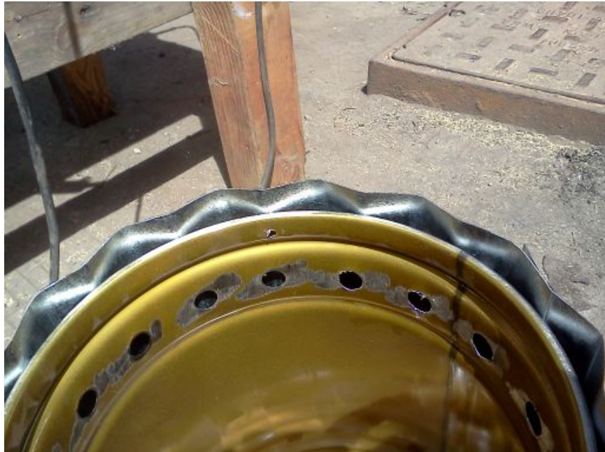
Roof Flashing on stove body
