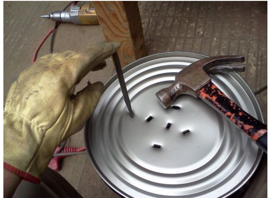
Chisel Primary Air Holes
