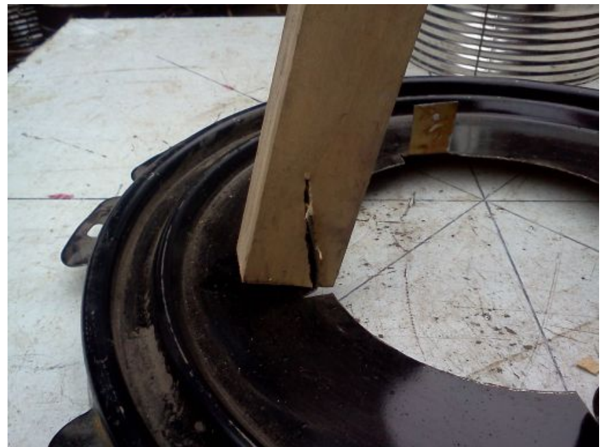
Bend Tab to a little more than 90 deg.
