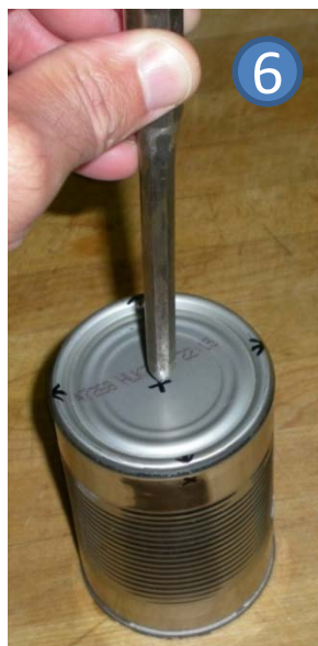
Mark a reference line about 1 inch from top for burner air inlets.
