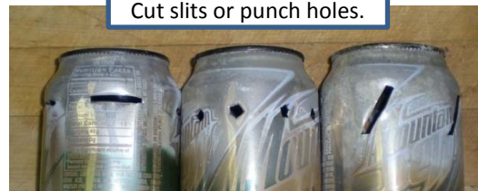
Alternate burner designs: Cut slits or punch holes.
