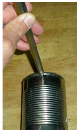
Punch air vent holes in the tin can.
