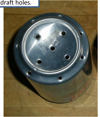
Carefully punch 12 to 15 vent/draft holes.
