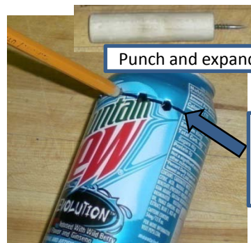
Alternate burner designs: Cut slits or punch holes.
