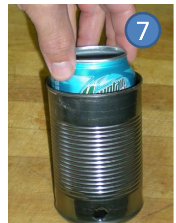
Assemble stove: nest cans by seating soda can snugly in/on bottom. The stove is now complete!
