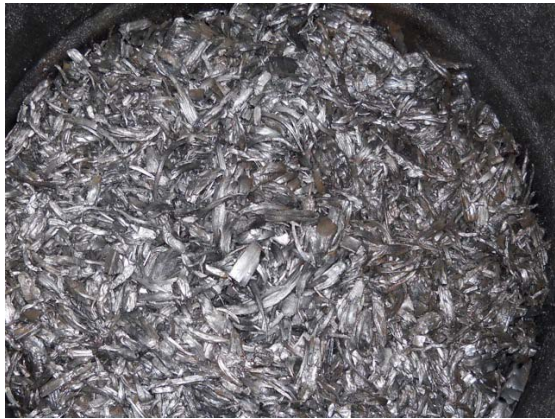
Figure 2 TLUD char (from shredded pallet wood)
