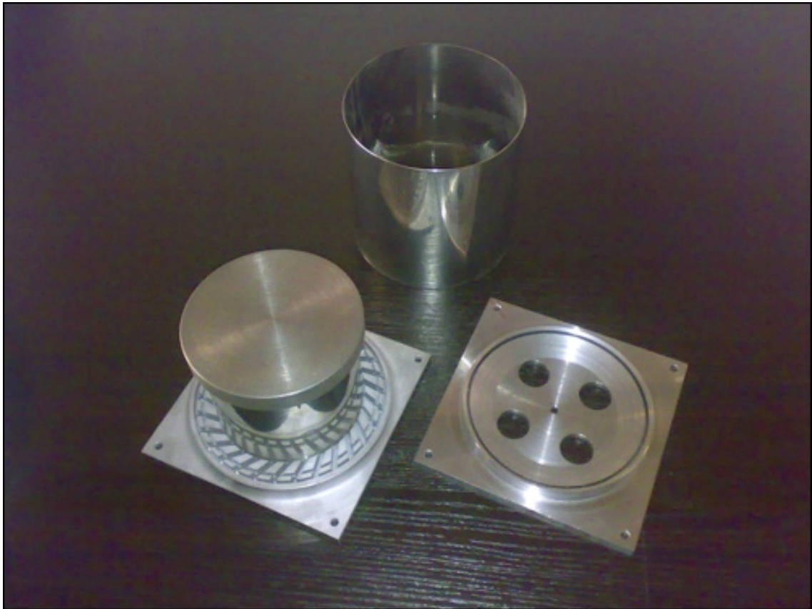
Figure A.9: The injection-molded components of the Lucia stove.
