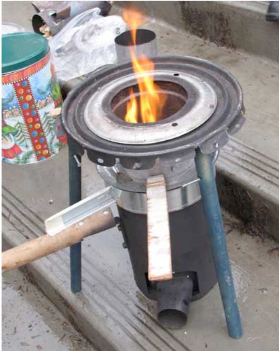
Figure A.5: A natural draft TLUD stove made from found materials.
