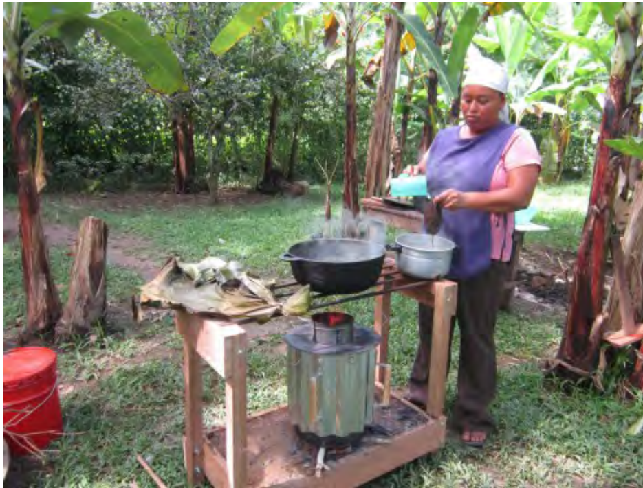
Cooking on the TLUD "Estufa Finca" in Costa Rica
