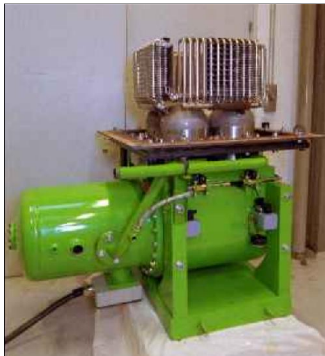
Figure 15. Stirling engine 35 kWe, before assembly. The heat transfer device is visible on the cylinder head.
