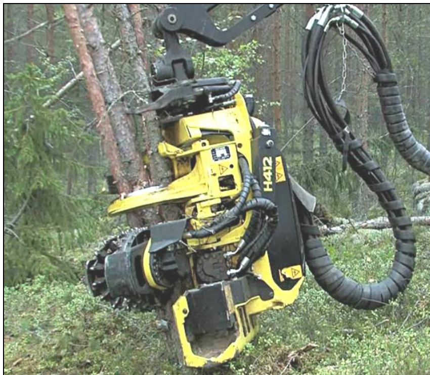
Figure 2. The MTH unit for multi-stem delimiting. Photo, John Deere ( www.deere.se )
