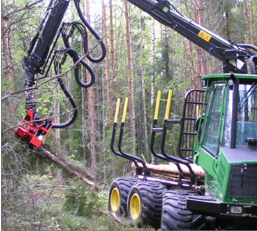
Figure 3. A crane-tip mounted scale for weighing of energy wood.
