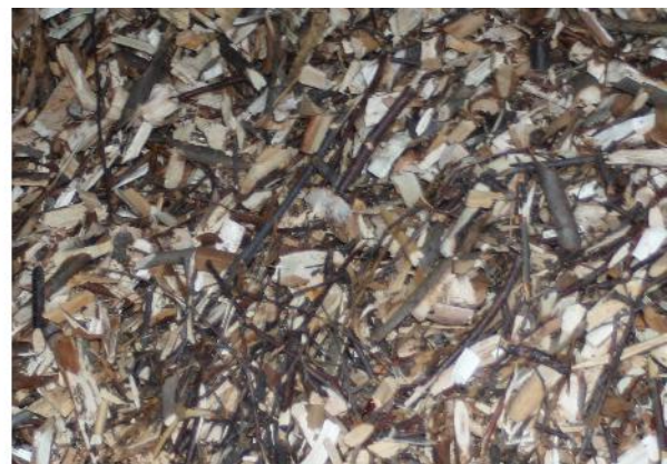
Uneven and poor wood chips.
