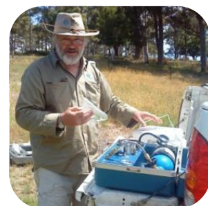
Garth Oliver measuring leaf water potential with a pressure chamber
