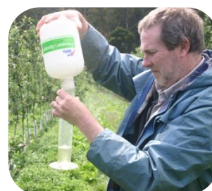
Steve Paterson collecting leachate from flux meters buried in the soil
