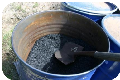
Biochar produced from Acacia green waste (sourced from Pacific Pyrolysis, NSW)
