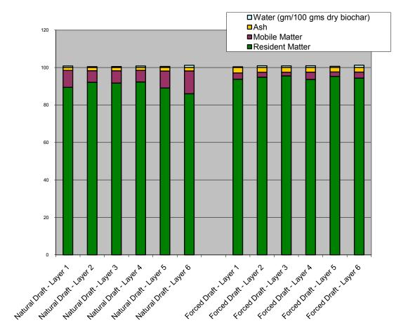
FIGURE 14: MODIFIED PROXIMATE ANALYSES OF TLUD CHARS
