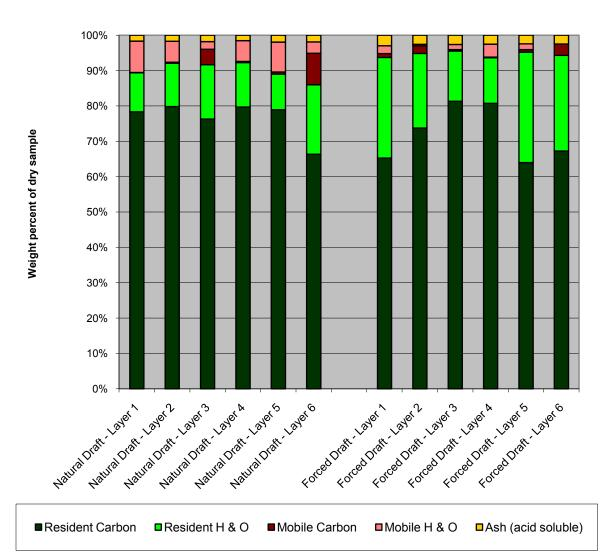
FIGURE 15: MODIFIED ULTIMATE ANALYSES OF TLUD CHARS
