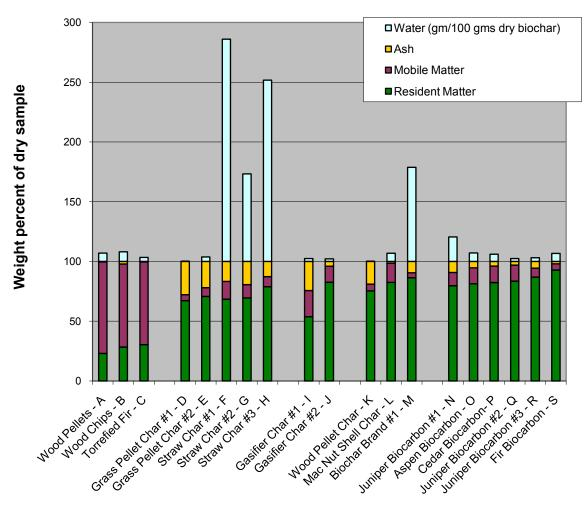
FIGURE 5: MODIFIED PROXIMATE ANALYSES OF CHARS
