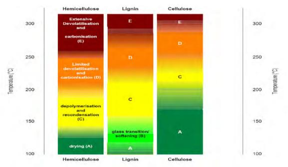
FIGURE 2: THERMAL MODIFICATIONS OF WOOD CONSTITUENTS
