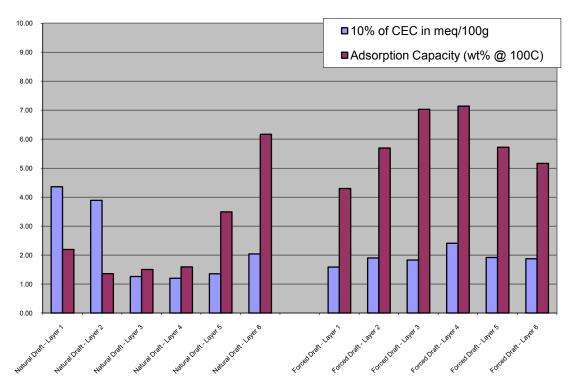
FIGURE 16: CEC AND ADSORPTION CAPACITY OF TLUD CHARS
