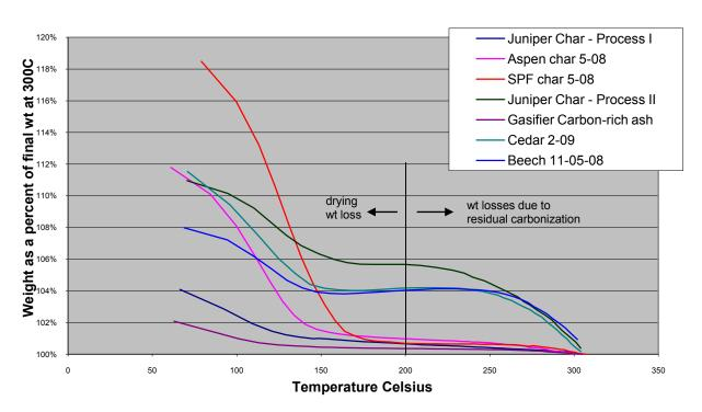
FIGURE 17: WEIGHT LOSS CURVES FOR A SET OF SEVEN CHARS
