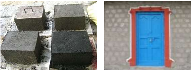
Picture 110 Biochar bricks and the building where biochar bricks were used in construction
