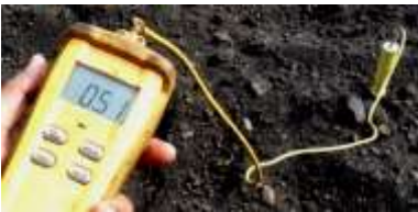
Picture 59 Higher temperatures indicate biochar compost is not complete. Below 37 degrees centigrade indicates that biochar compost is ready for application
