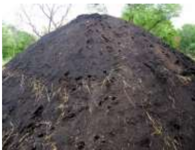
Picture 35 Charcoal being produced by traditional earth mound kiln method
