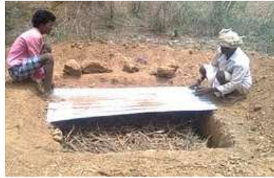
Picture 37 Biochar being produced by pit kiln method
