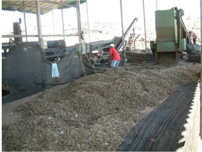
Crushed plastic for feeding the gasifier
