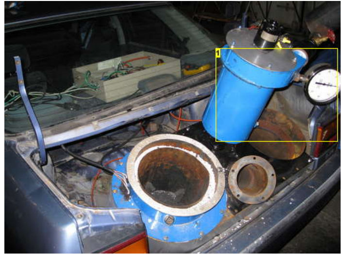
Image Notes 1. gas filter unit with pressure sensor
