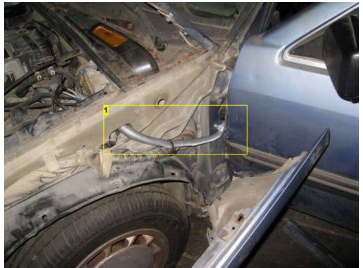
Image Notes 1. wiring from the RCU to the engine area
