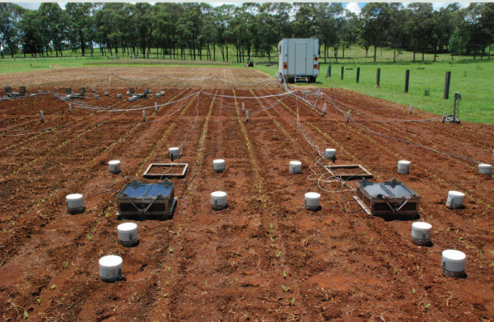
FIGURE 3.3: Greenhouse gas chambers measure carbon dioxide, nitrous oxide and methane continuously in the field. Photo: Lukas Van Zwielen
