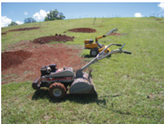
FIGURE 5.10: Hand-driven rotary hoe for biochar incorporation. Photo: Josh Rust
