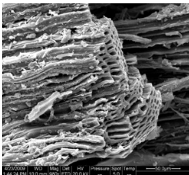
FIGURE 4.5: Scanning electron microscope image of wood waste biochar. Note the original internal structure. Photo: Adriana Downie
