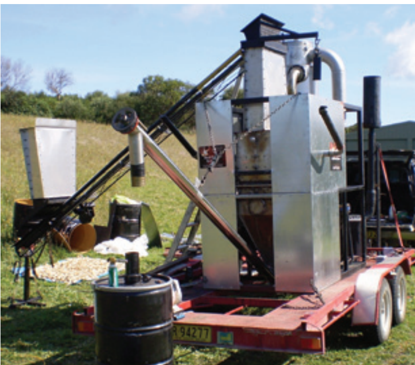
FIGURE 2.7: Portable 200kg/hr biomass gasification module for biochar and clean fuel gas production. Photo: Peter Davies, Real Power Systems P/L
