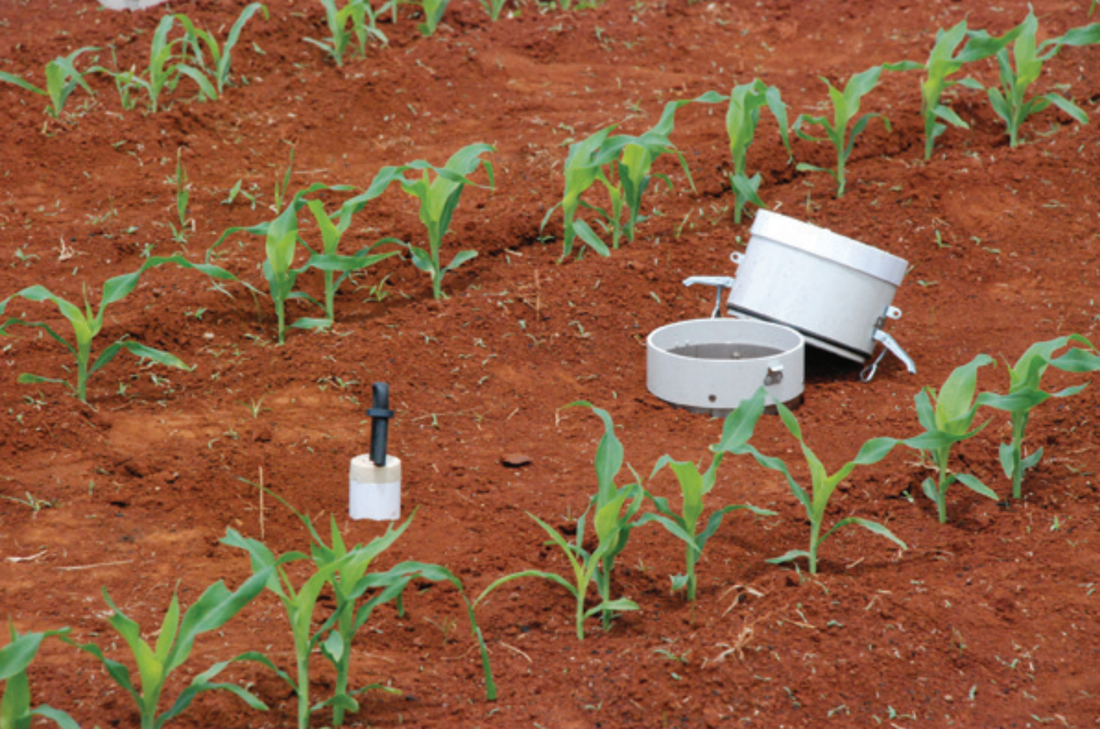
FIGURE 7.2: PVC tube greenhouse gas chamber inserted into the soil to monitor greenhouse gases. Photo: Josh Rust
