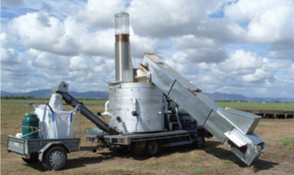
FIGURE 2.5: BiGchar 1800 equipment set up for mobile in field processing of sugar cane trash. Photo: James Joyce
