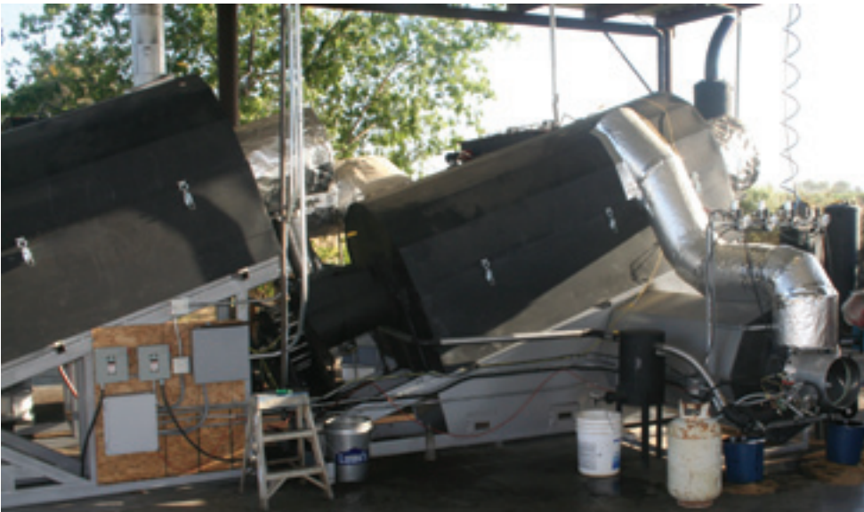
FIGURE 2.6: Biochar-Energy Systems' single module continuous slow pyrolysis unit. Photo: Russell Burnett
