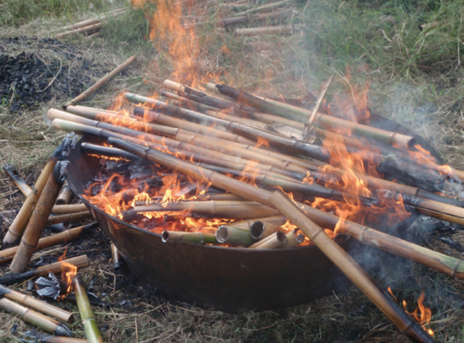
FIGURE 2.2: These bamboo lengths are combusting on the surface before collapsing into a zone of pyrolysis below. Photo: Lukas Van Zwieten
