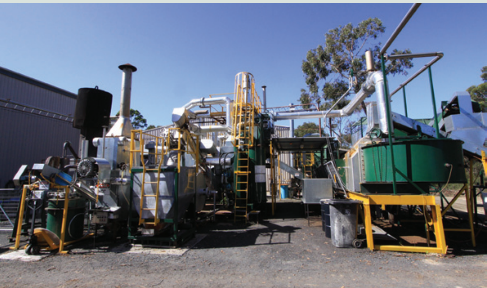
FIGURE 2.4: Pilot commercial pyrolysis unit based at Somersby, NSW, owned and operated by Pacific Pyrolysis. Photo: Adriana Downie
