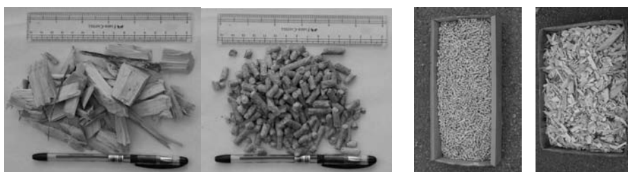
Fig. 9. Wood chips and wood pellets tested in the JRB-1 gasifier.
