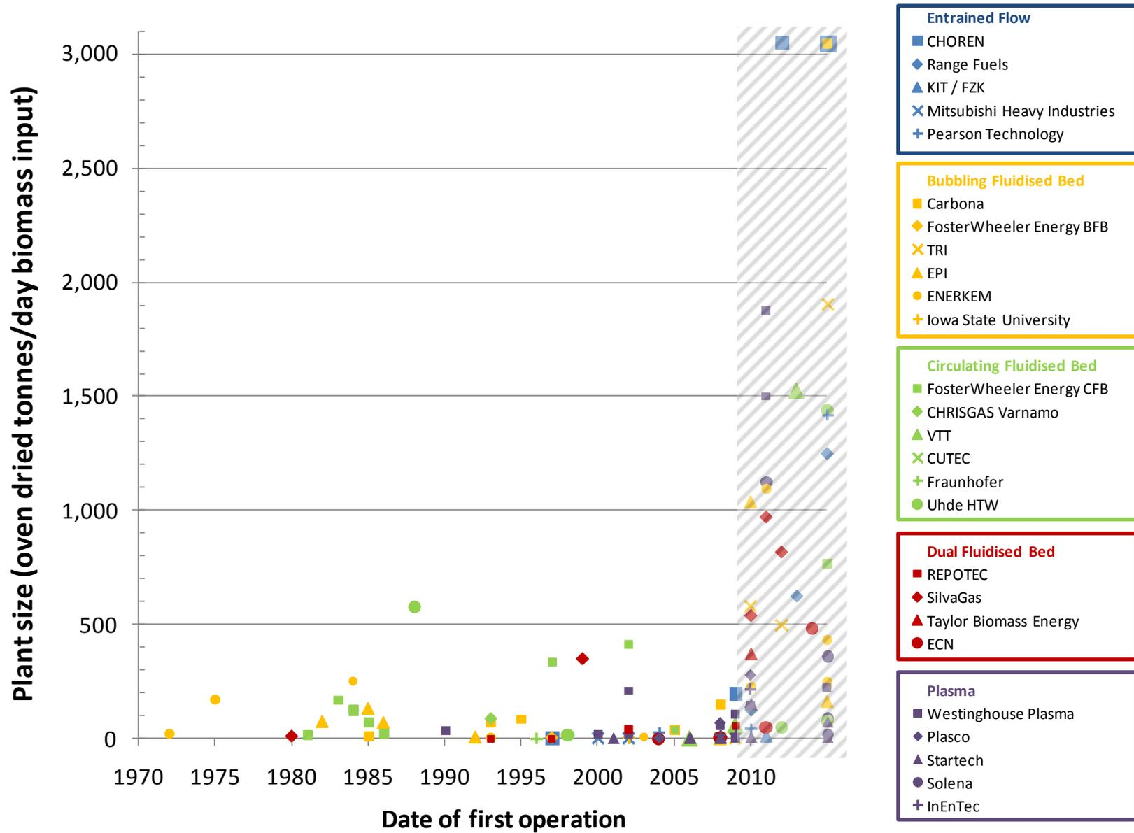
Figure 3: Biomass gasification plant size and year of first operation. The size given is for the whole plant biomass input (the total of all gasifier modules)
