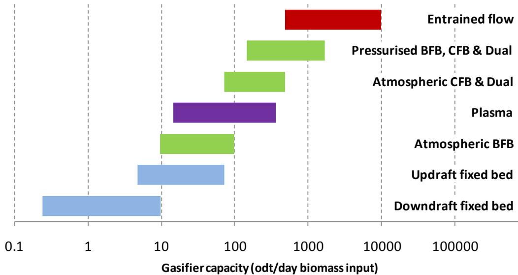
Figure 1: Gasifier technology capacity range<sup>24</sup>
