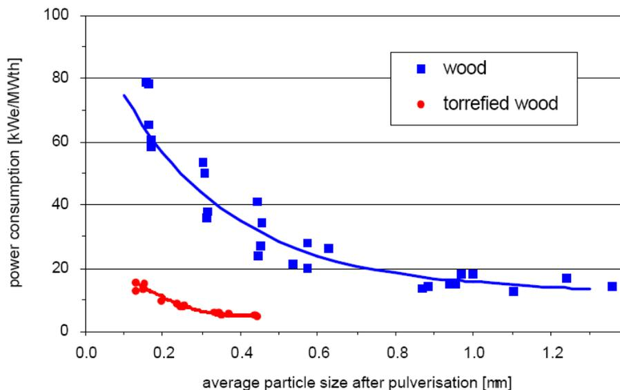
Figure 2: Milling power consumption vs. required particle size<sup>42</sup>
