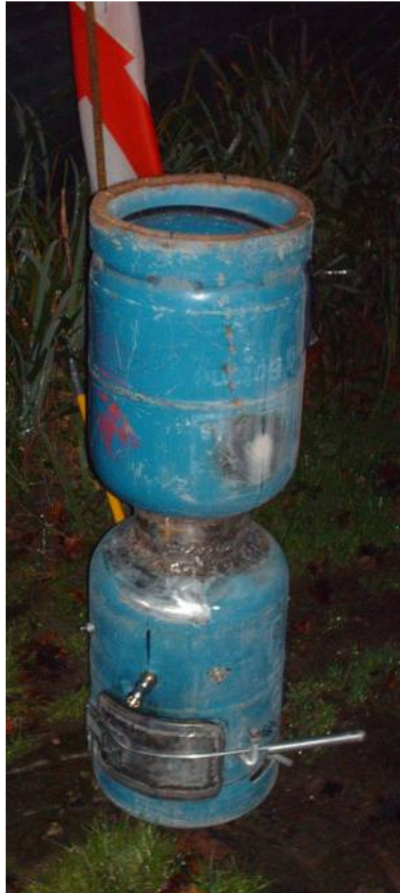
Basic gasifier unit.
