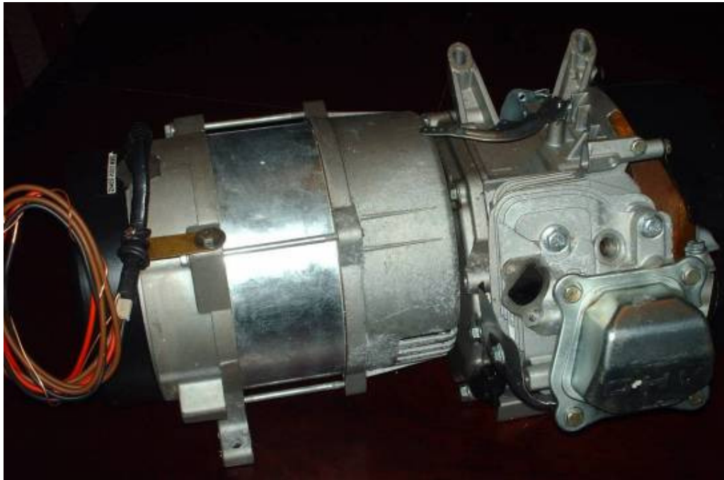
The donor ICE and 2.2Kw generator.
