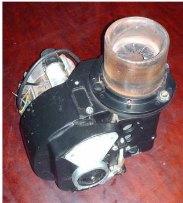
A salvaged blower from a oil fired boiler. The oil pump has been removed and the hole left will become the woodgas inlet. There's a 240v motor on this, not sure what to do yet with this.
