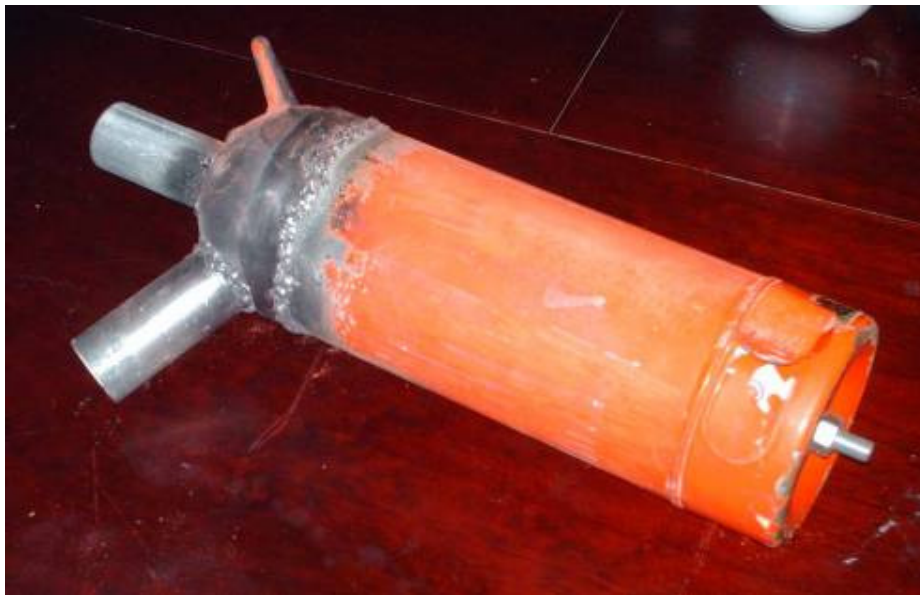
Initial Primary Filter made from old fire extinguisher.
