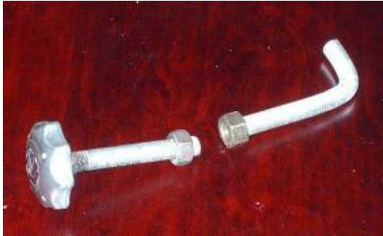
Grate Shaker handle and grate link.
