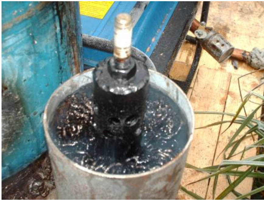
Top off Primary filter showing SS scrubber pads. Gas flow is up through pads, then down through centre.
