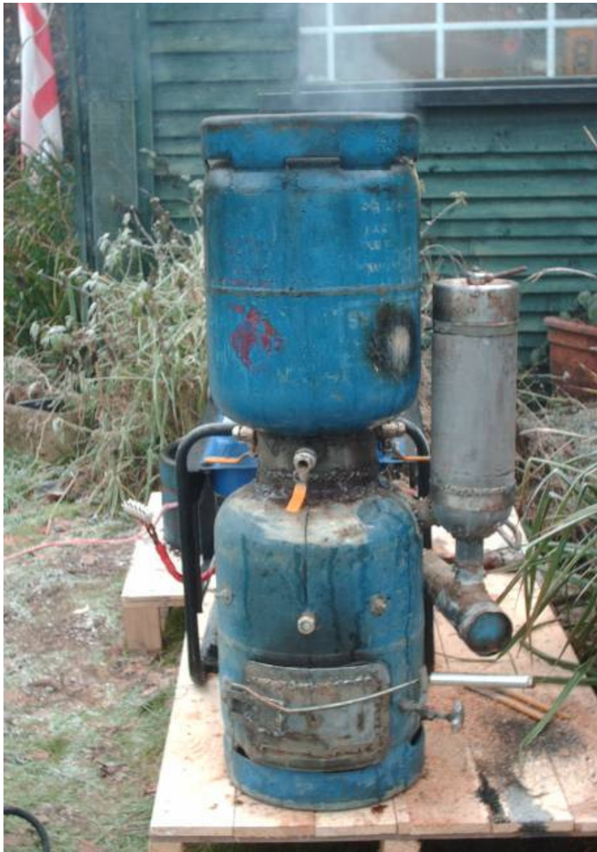
The fire lit, blower switched on and door sealed shut.
