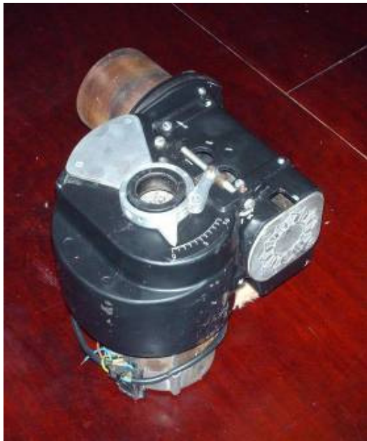
A salvaged blower from a oil fired boiler. The oil pump has been removed and the hole left will become the woodgas inlet. There's a 240v motor on this, not sure what to do yet with this.
