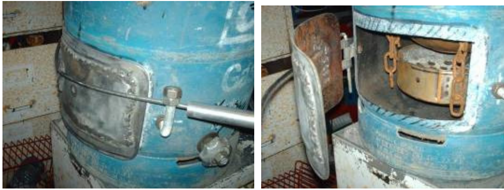
Spring fit door awaiting door seals. Grate can be seen hung by chains.
