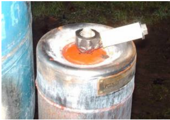
Filter top nut with tightening handle welded on.
