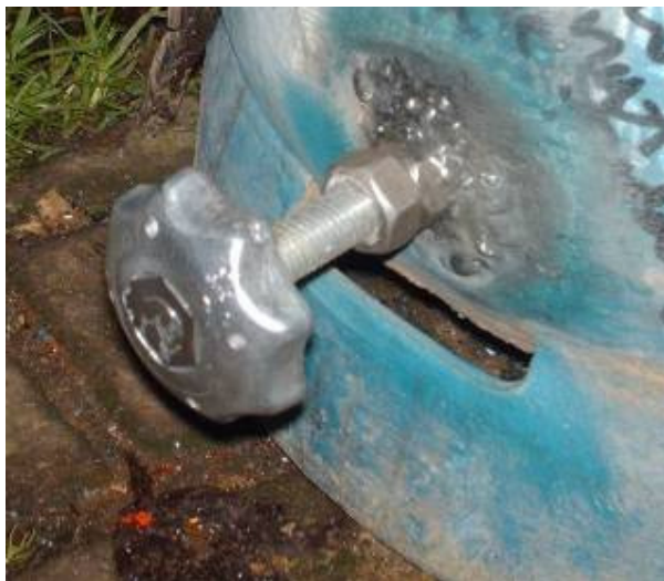
The Shaker stud is kept long for heat insulation.
