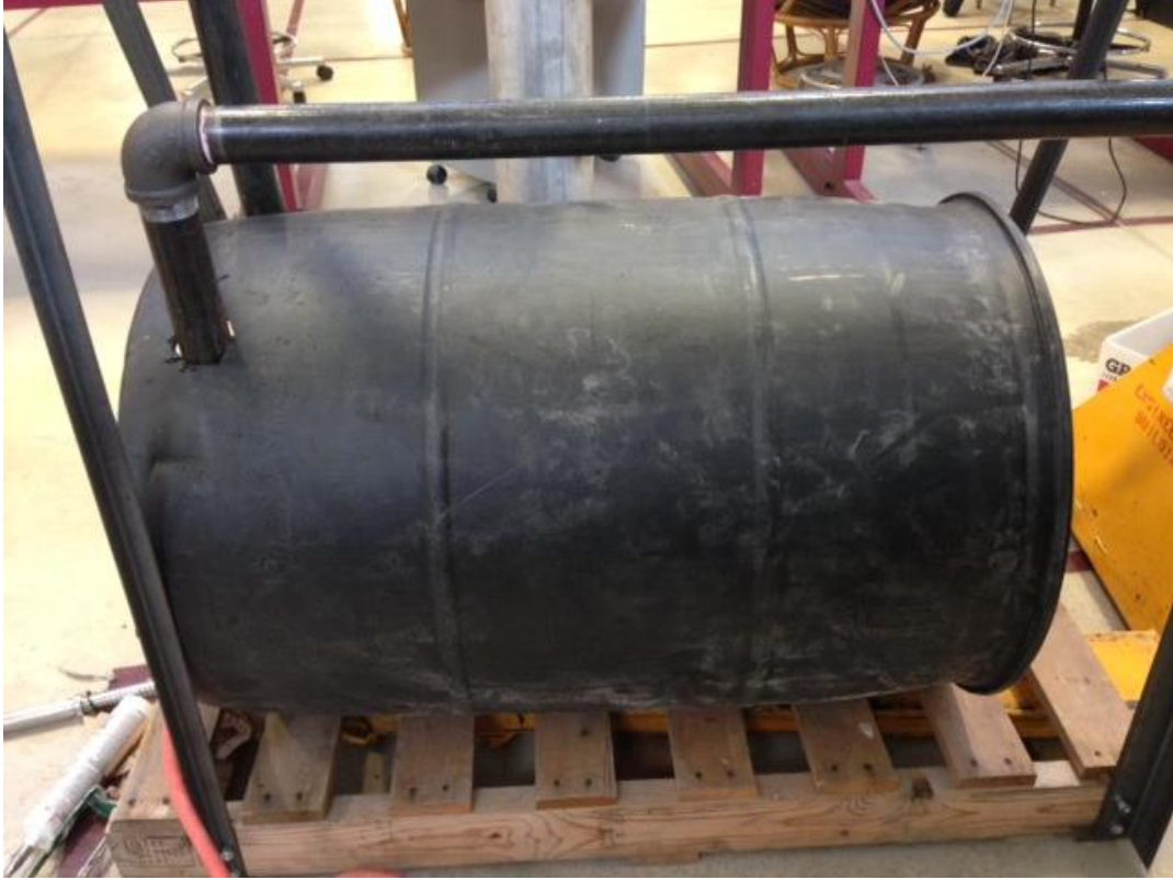
Figure 2-7 Steam Feed Heat Exchanger Exterior
