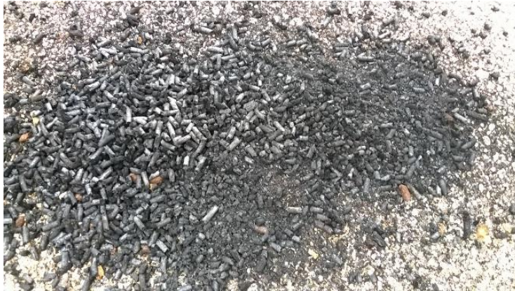
Figure 4-3 Charred Pellets and Ash Observed in Gasifier Disassembly
