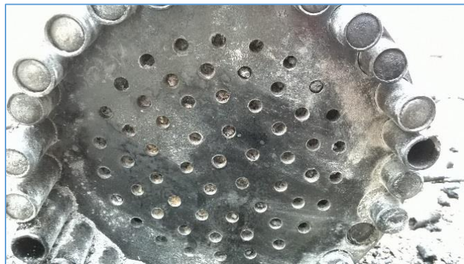
Figure 4-2 Plugged Ash Grate Observed in Gasifier Disassembly
