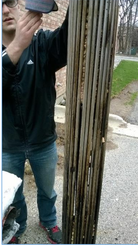
Figure 4-1 Evidence of Bridging in Gasifier Disassembly
