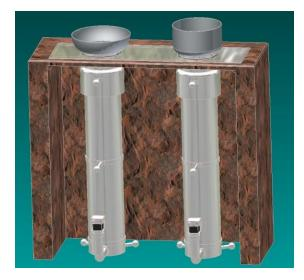
someone to accidently knock over the gasifier. With an enclosure, pots and pans are not supported by the gasifier, but by the burner grate on the top of the enclosure. An enclosure can be inexpensively constructed out of brick or stone (see picture above).
