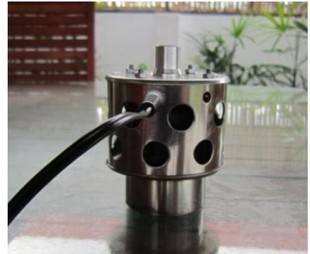
In the original Belonio design, the fan was permanently attached to the reactor. But now the fan can be detached from the reactor when it is being emptied of biochar. In this way, rising hot air does not damage the fan when the reactor is turned upside down.
