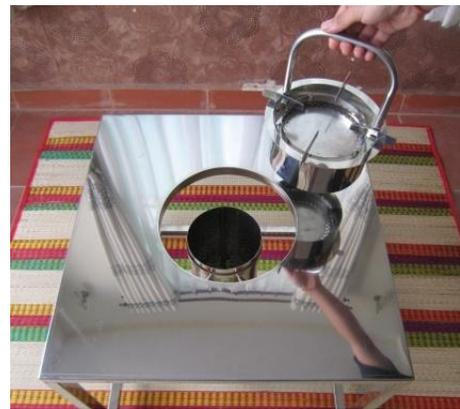
The top of the enclosure can be made out of [terrazzo](#) at a cost of about 10 US dollars. Or it can be made simply by cutting a hole in a large [ceramic floor tile](#). Here the cost drops down to \$2.50 US dollars. The small 100 pellet gasifier set within an enclosure with a ceramic table top looks like [this](#). The 150 gasifier set with an enclosure with a ceramic table top looks like [this](#).
