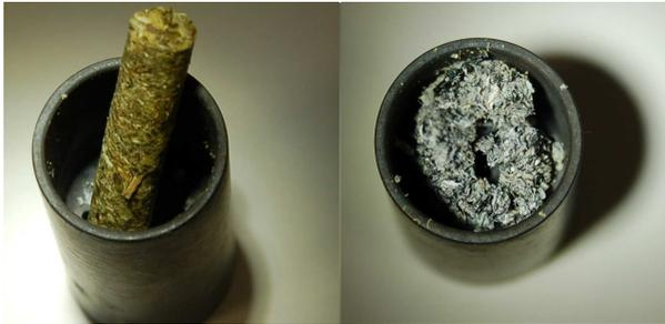
Figure 5.12: Pellet before (left) and after (right) gasification and combustion in the reactor grate
