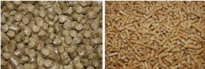
Figure 4.14: *Fuel pellets as received, left picture: grass 16 mm/ right picture: wood 6 mm*
