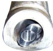
Figure 4.5: *Tip of the auger showing a drill hole for less heat transport into the fuel pipe.*
