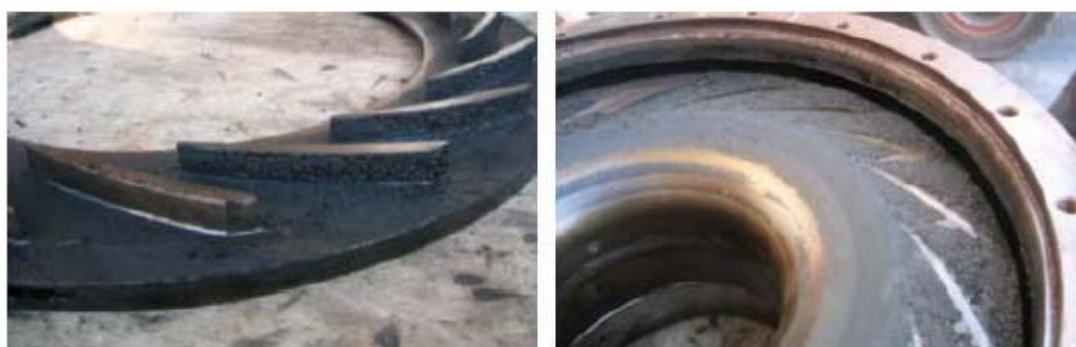
Figure 7-6: Deposits of coke and tar components in the diffuser housing, [55]
