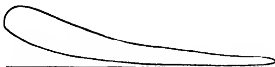
FIG. 56. Defective indicator power diagram due to bad gas or wrongly adjusted mixture of gas and air.
