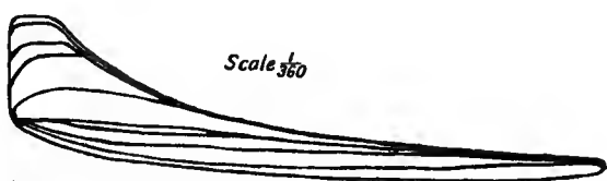
FIG. 70. Indicator diagrams taken while changing from 'no load' to 'full load.'
