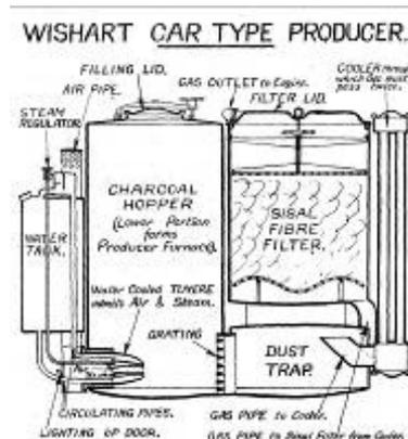
Wishart Car Type Gas Producer (Blackburn, Victoria). They were manufacturing units before 1938 and had developed an ingenious automatic device to control the amount of water added.
