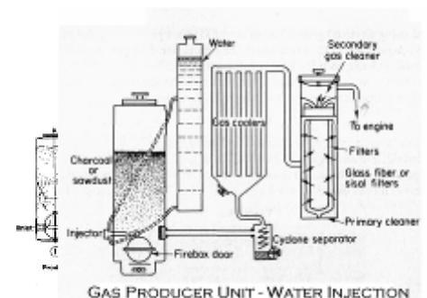
The weight of the typical GPU was between 400-500 lbs (empty) for a passenger vehicle unit. Add another 50-100 lbs for the charcoal.
