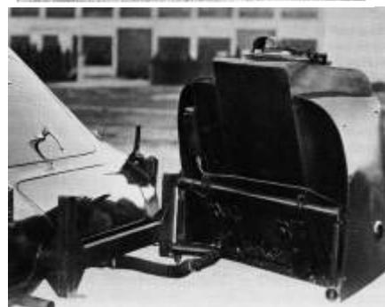
The Grieg Gas Producer (Power Gas Co Pty Ltd of Melbourne).
