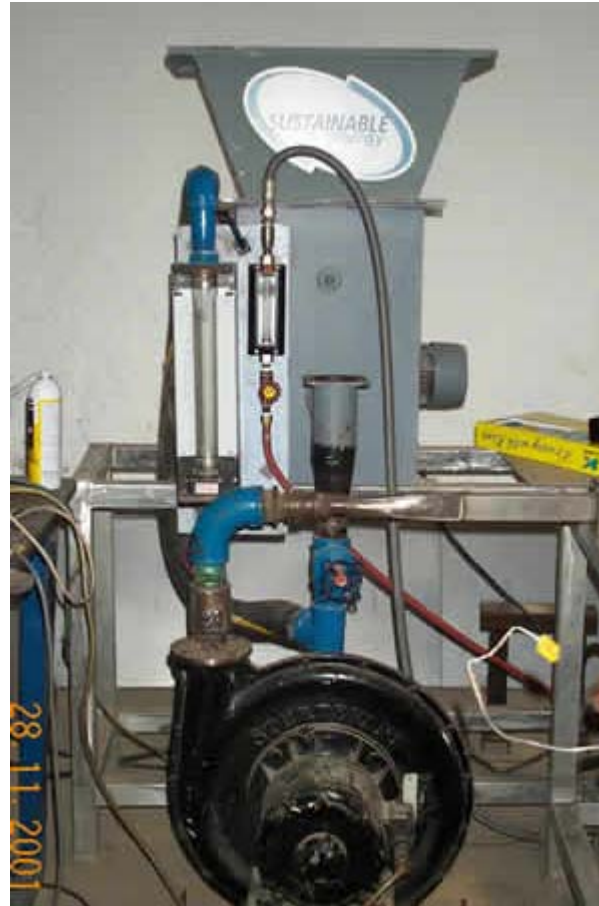
Figure 4 Sawdust hopper and feeder system
