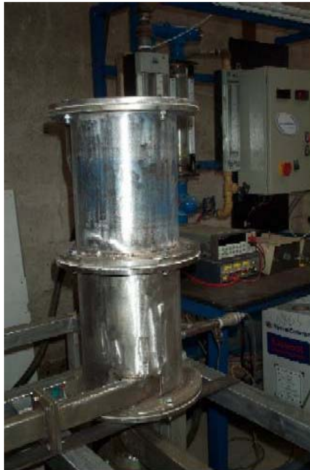
Figure 3 Cyclone gasifier without insulation and outer jacket
