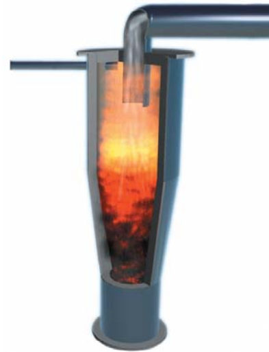
Figure 7.3. Schematic of a cyclone gasifier (reproduced courtesy of MEVA Innovation).
