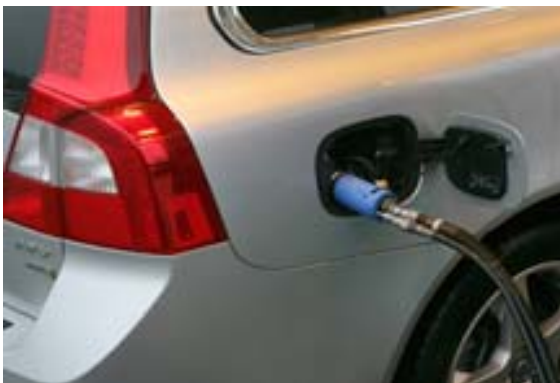
Figure 6.1. The Volvo V70 AFV BI-FUEL is a typical gas fuelled car (courtesy of AFV) [3].
