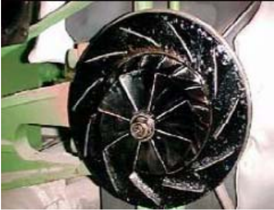
Figure 6.19. Tars condensed on a compressor wheel (courtesy of GE's Jenbacher gas engine business) [19].
