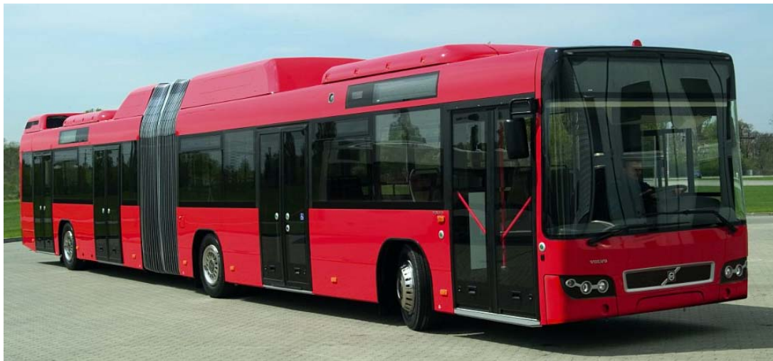
Figure 6.2. Biogas-fuelled city bus. The gas tanks are placed on the roof (courtesy of Volvo).
