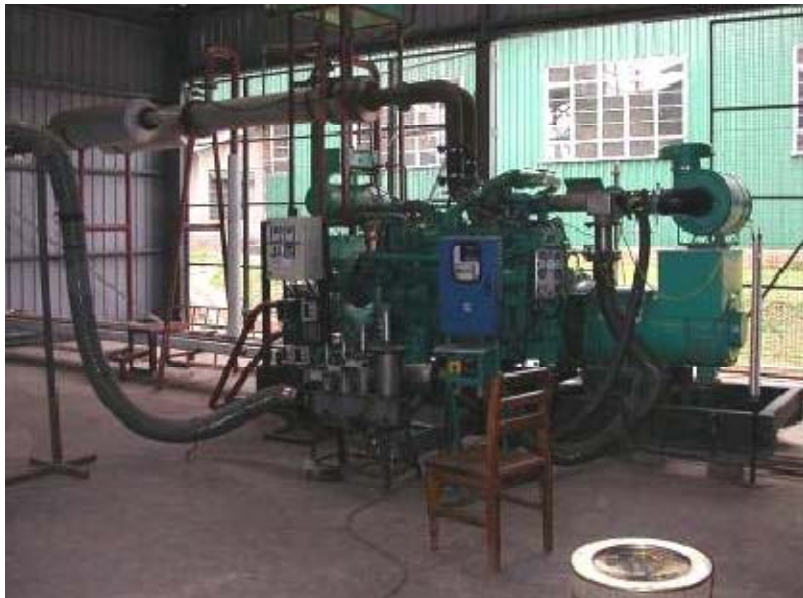
Figure 7.18. The 250 kW syngas engine with heat exchanger (photo courtesy of T. Buchholz).
