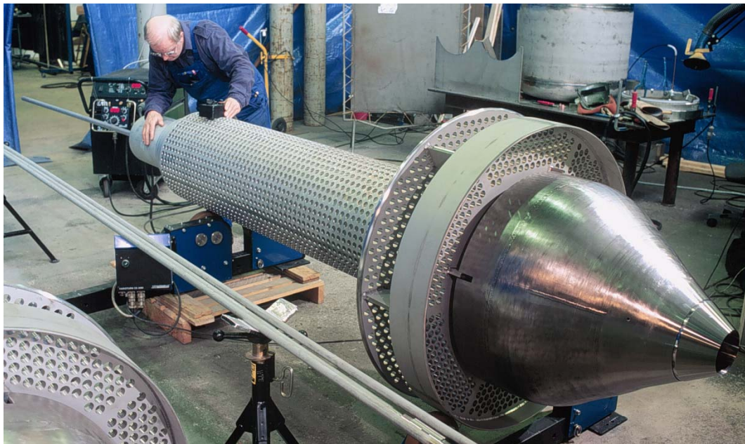
Figure 5.7. The Topsoe CTS burner for ATR (courtesy of Haldor Topsoe A/S, DK).
