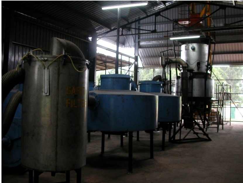
Figure 7.17. The filter line and the WBG 400 gasifier (photo courtesy of T. Buchholz).
