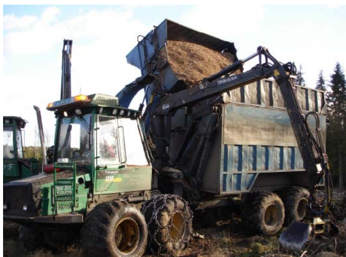
Figure 2.8 Chipping machine emptying its load into the tractor for transportation to large containers. (photo reproduced by courtesy of Johan Andersson)
