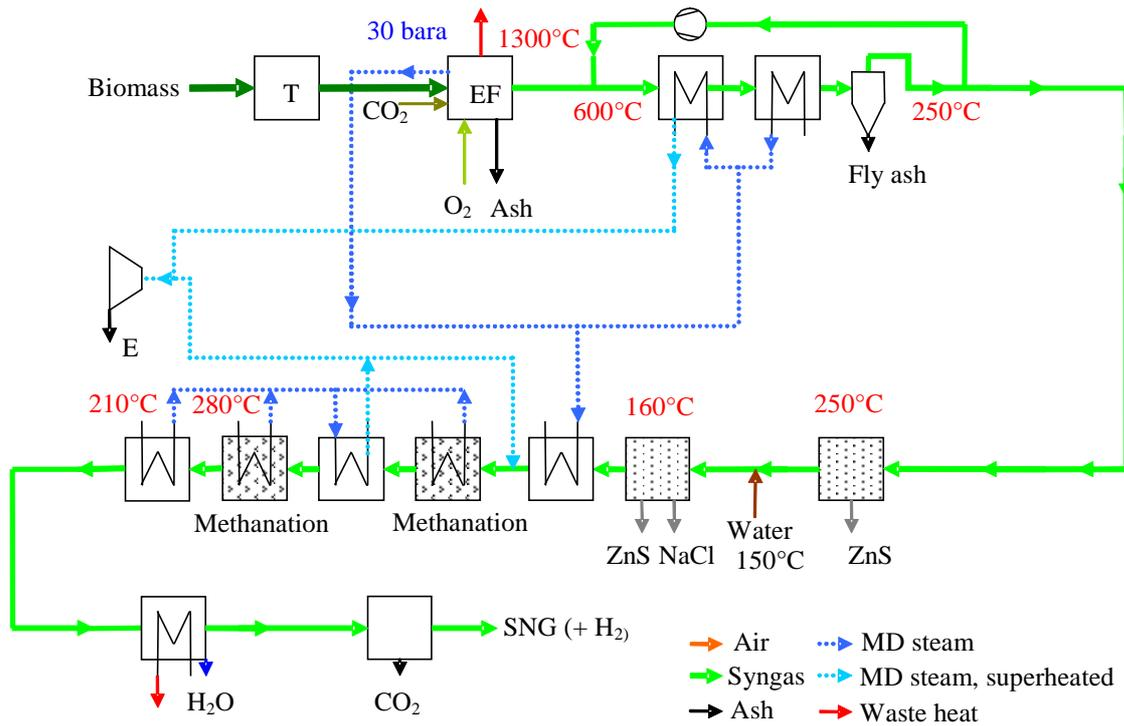
Figure 4-2: Scheme of EF SNG system.
