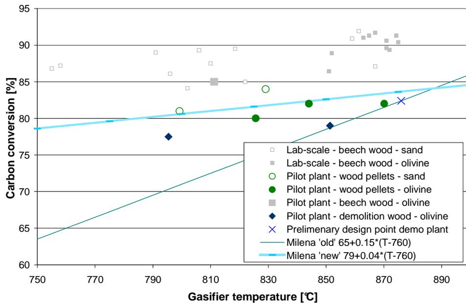
Figure 7-6: Measured carbon conversions in MILENA lab-scale and pilot plant.
