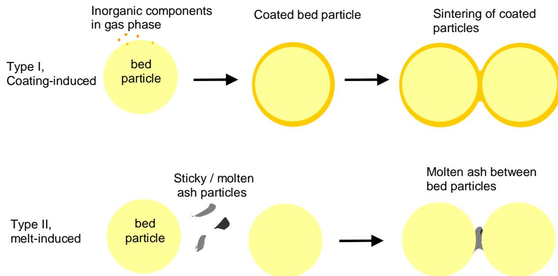
Figure 2-4: Basic principles for type I and type II bed agglomeration
