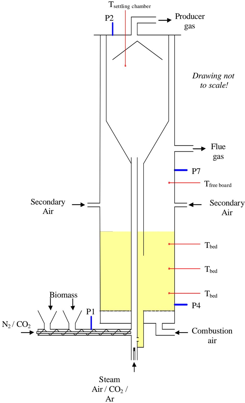
Figure 6-8: MILENA lab-scale gasifier.
