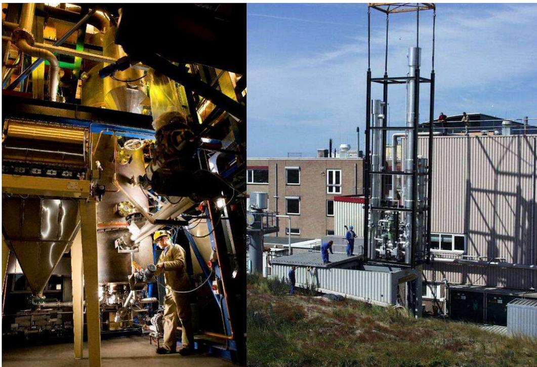
Figure 6-1: pilot-scale MILENA gasifier (left) and installation of the OLGA pilot-scale gas cleaning (right) at ECN.
