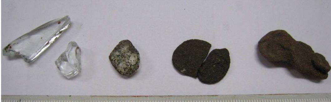
Figure 7-26: Various stages of bed material covering of glass particles.
