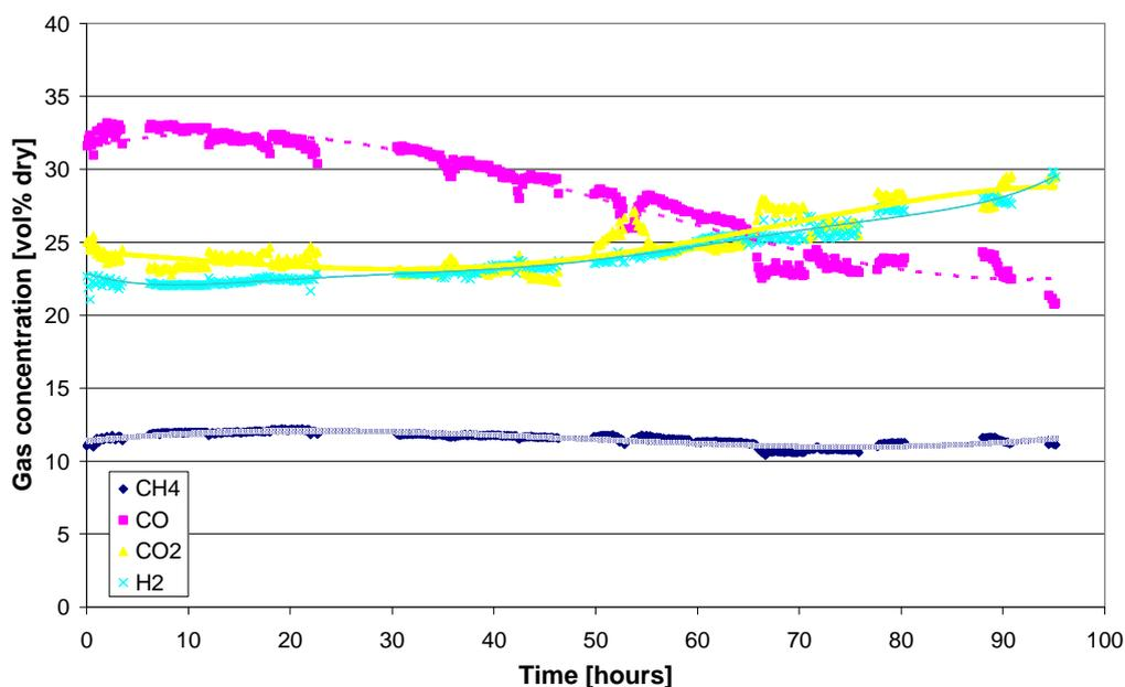
Figure 7-22: MILENA lab-scale duration test gas composition.
