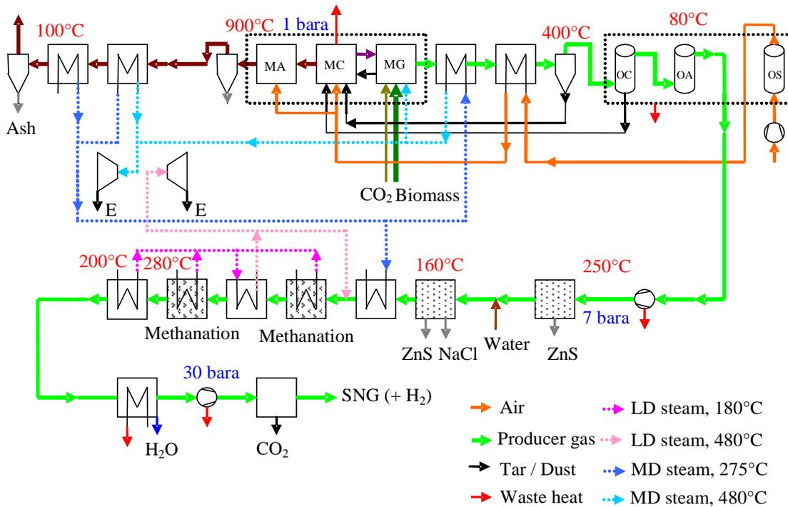
Figure 4-4: Scheme of Indirect gasifier SNG system.
