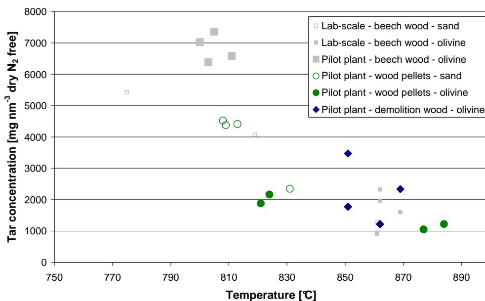
Figure 7-16: Concentration of class 2 tars as function of temperature.
