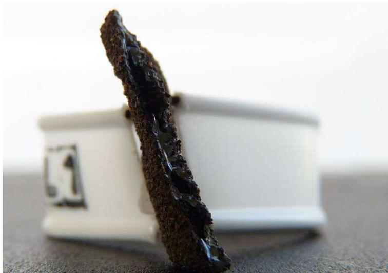
Figure 7-25: Close-up of broken glass particle.
