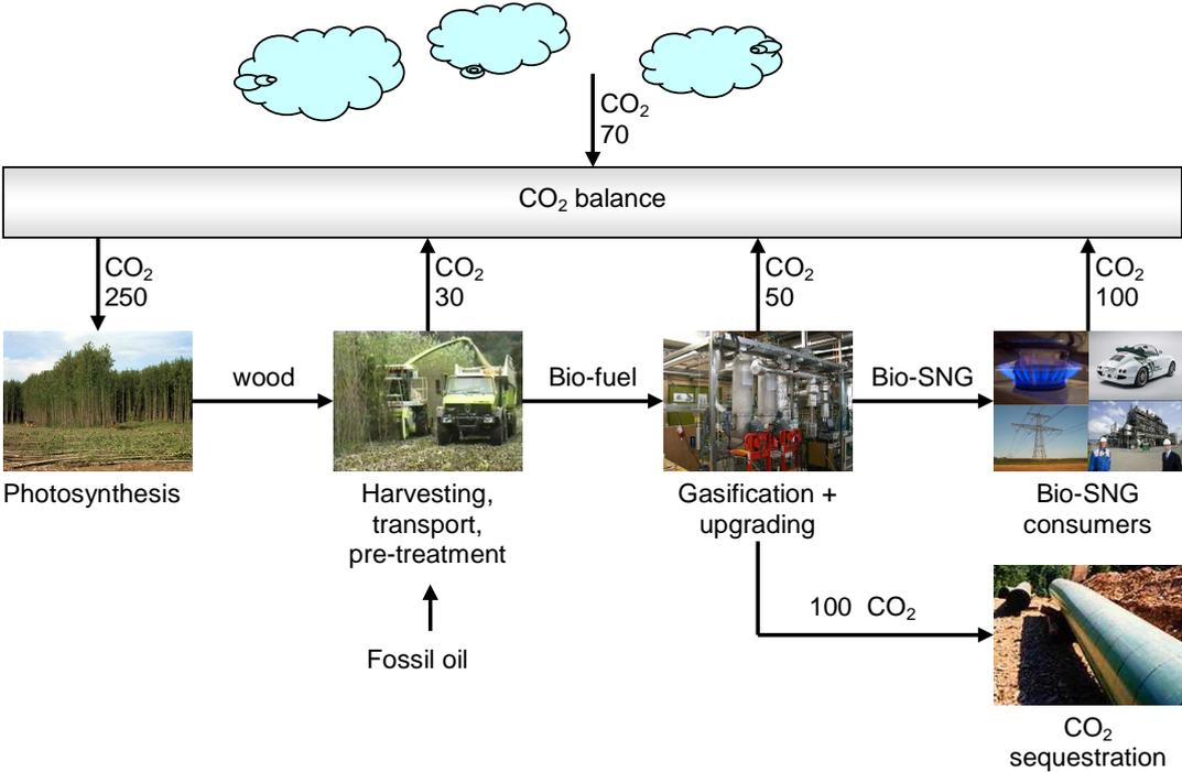
Figure 1-1: Indicative CO<sub>2</sub> balance for Bio-SNG system based on MILENA gasification.
