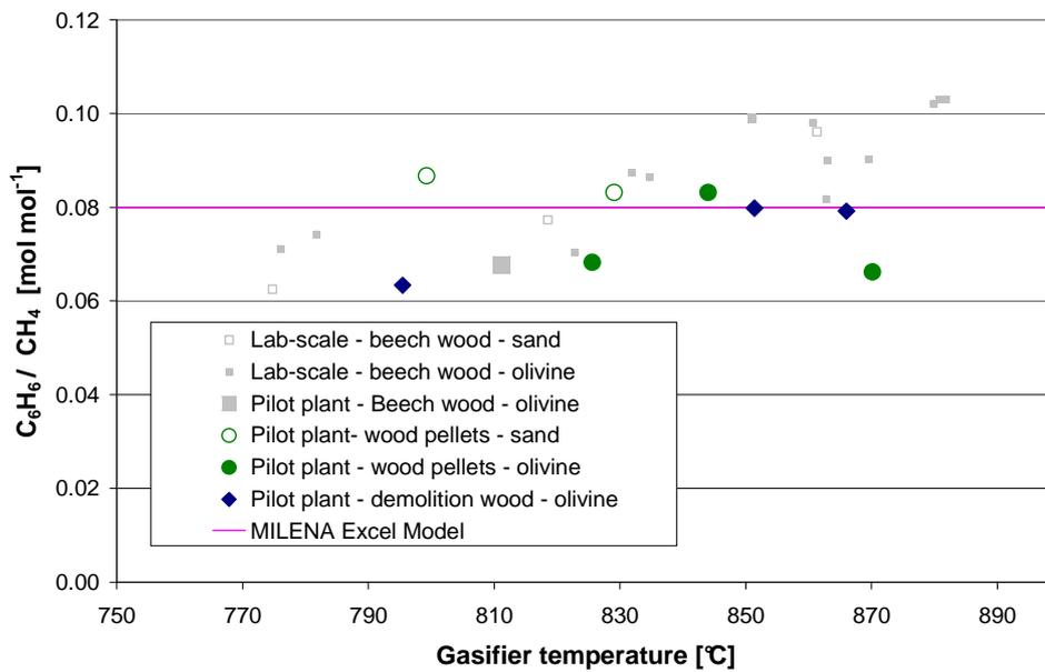
Figure 7-12: C<sub>6</sub>H<sub>6</sub> yield relative to CH<sub>4</sub> as function of temperature.
