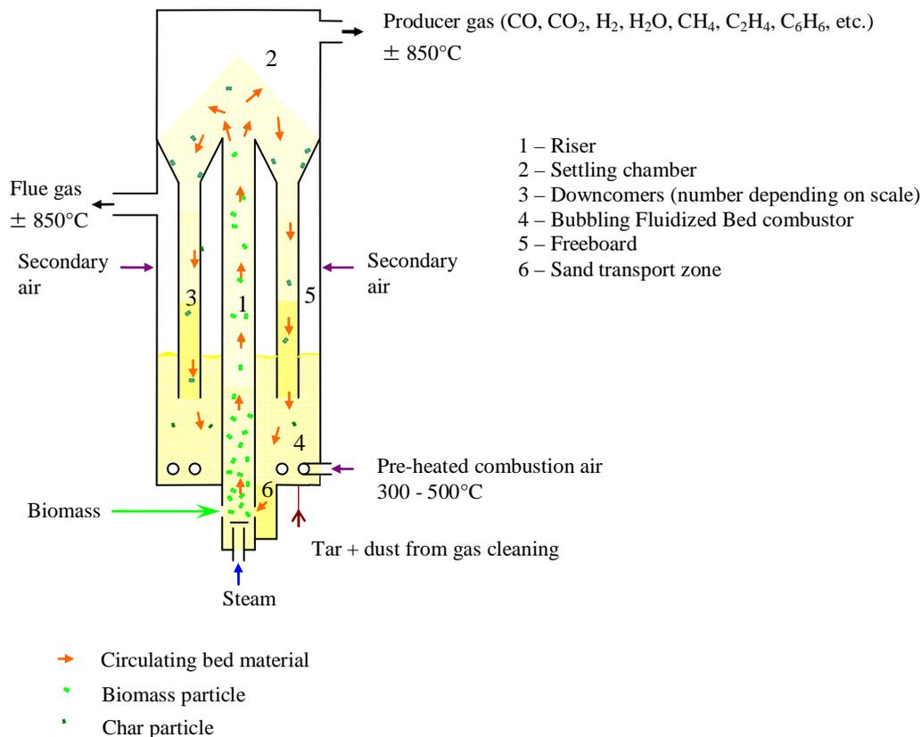
Figure 2-5: Simplified scheme of MILENA gasification process.
