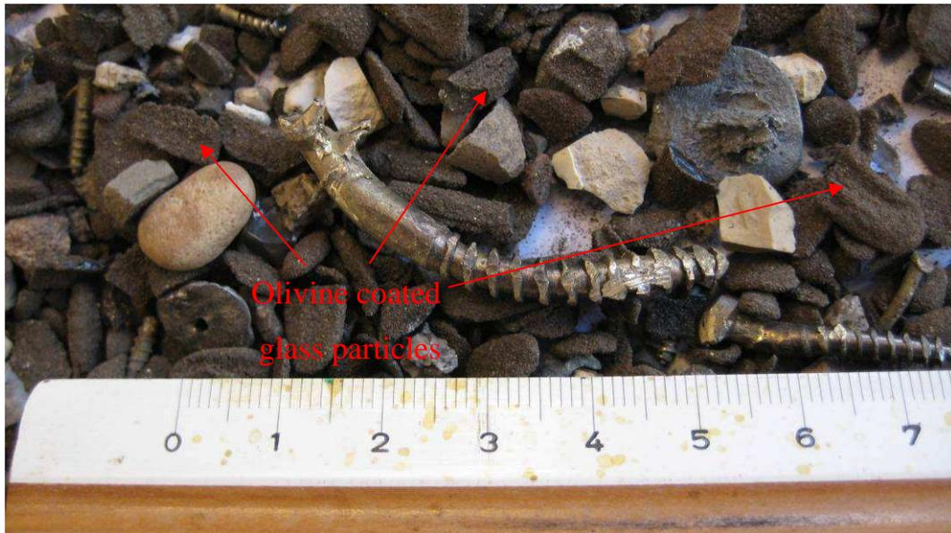
Figure 7-24: Bottom ash riser, produced during demolition wood B test.
