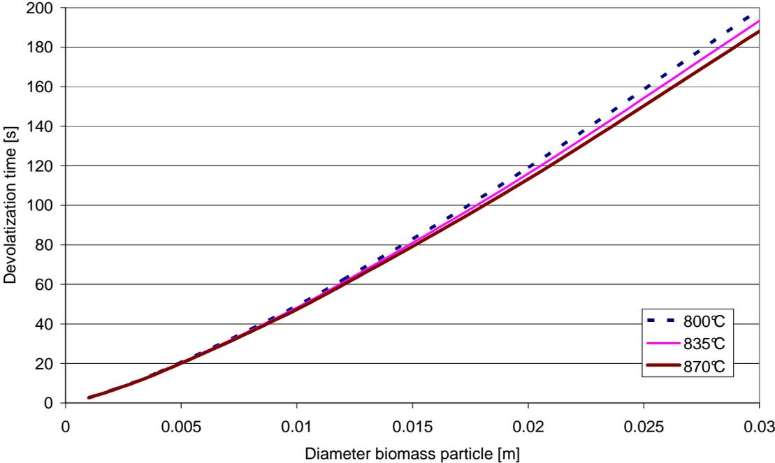
Figure 6-2: Calculated devolatilization times assuming spherical particles.
