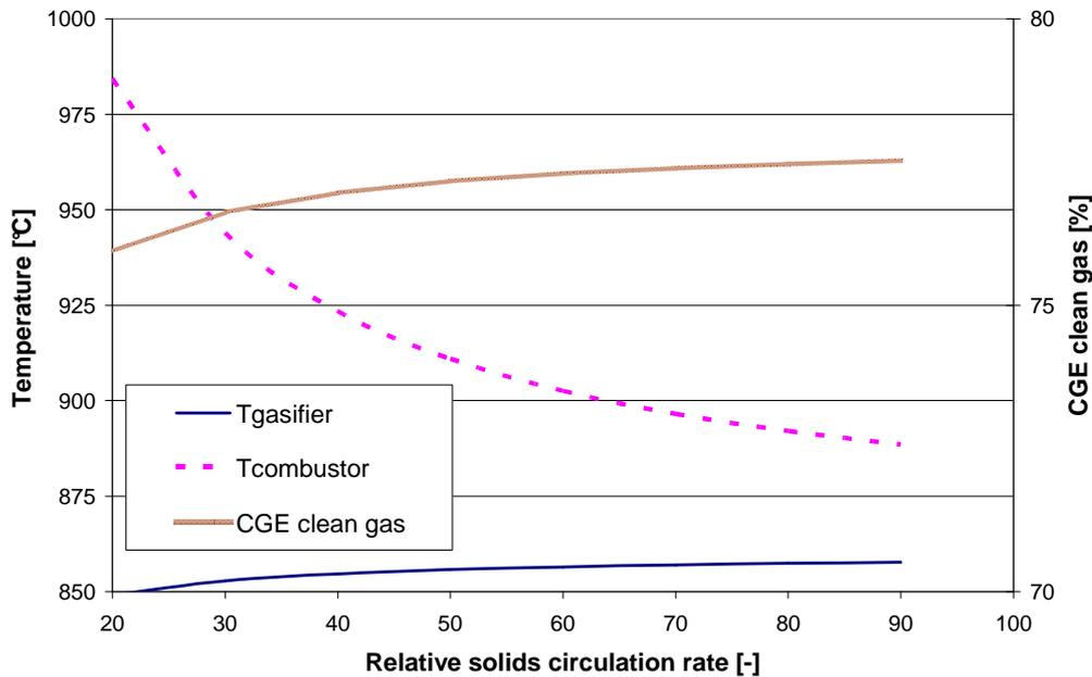
Figure 7-2: Effect of relative solids circulation rate (defined as mass flow solids per mass flow biomass on a.r. basis) on reactor temperatures and CGE.
