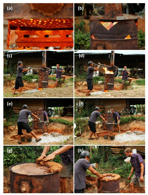
Photo series showing shutdown procedure: When bottom of drum begins to glow (a) and blue flames appear in crown (b) then pyrolysis is nearing completion. Remove the crown and chimney (c) and (d). Put on the lid and move the reactor body to the adjacent mud pit to seal the bottom (e) and (f). Seal the top with mud to prevent air leaks (g) and (h). (Photography by Lyse Kong.)
