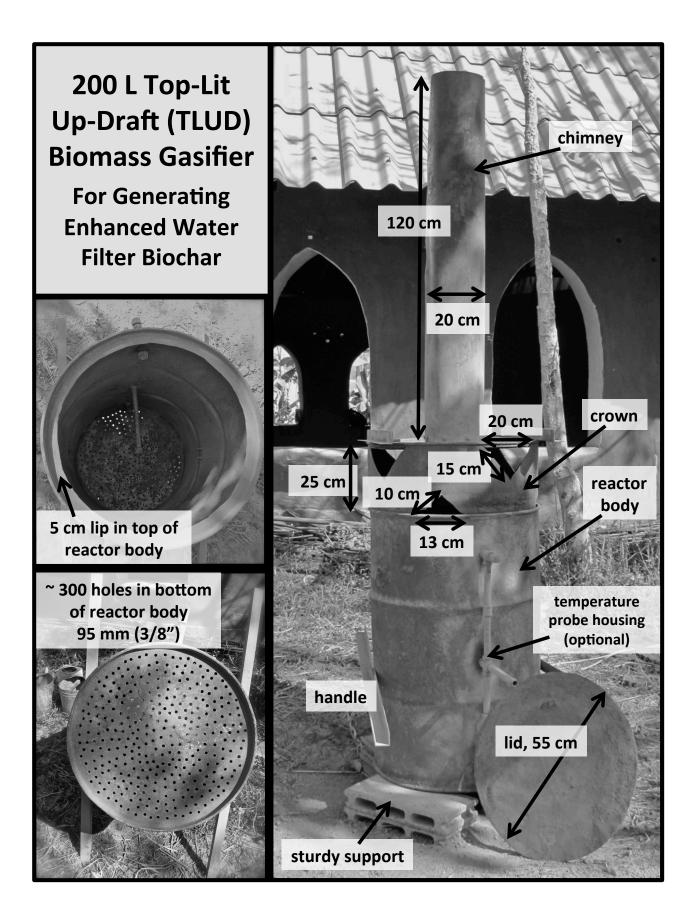
An instructional video explaining the conceptual background, construction, and operation of this unit can be accessed from the Aqueous Solutions website: www.aqsolutions.org.
