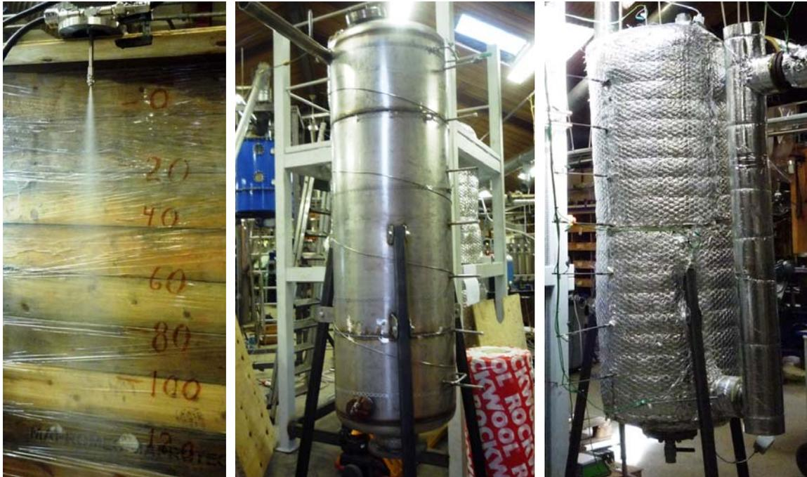
Figure 4.4 Test of nozzle (left), evaporative cooler without insulation (centre) and evaporative cooler with insulation (right)
