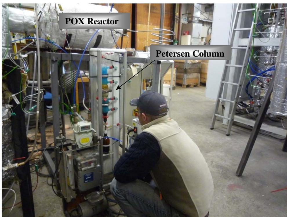
Figure 4.10 *Partial oxidation (POX) and tar sampling setup*
