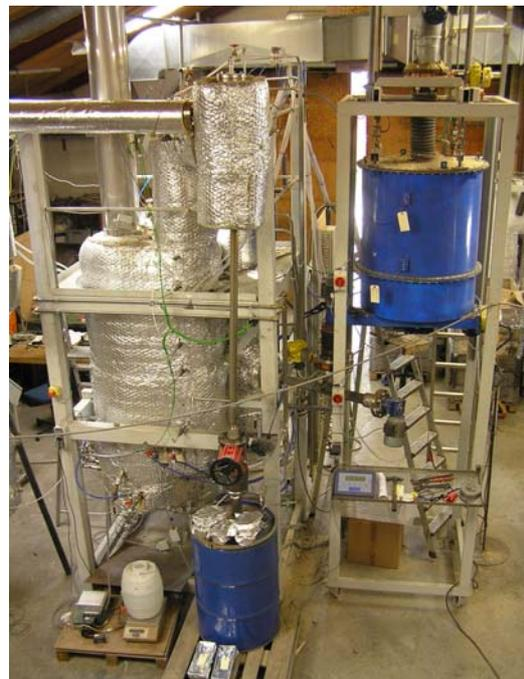
Figure 2.14 100 kW<sub>th</sub> LT-CFB gasifier
