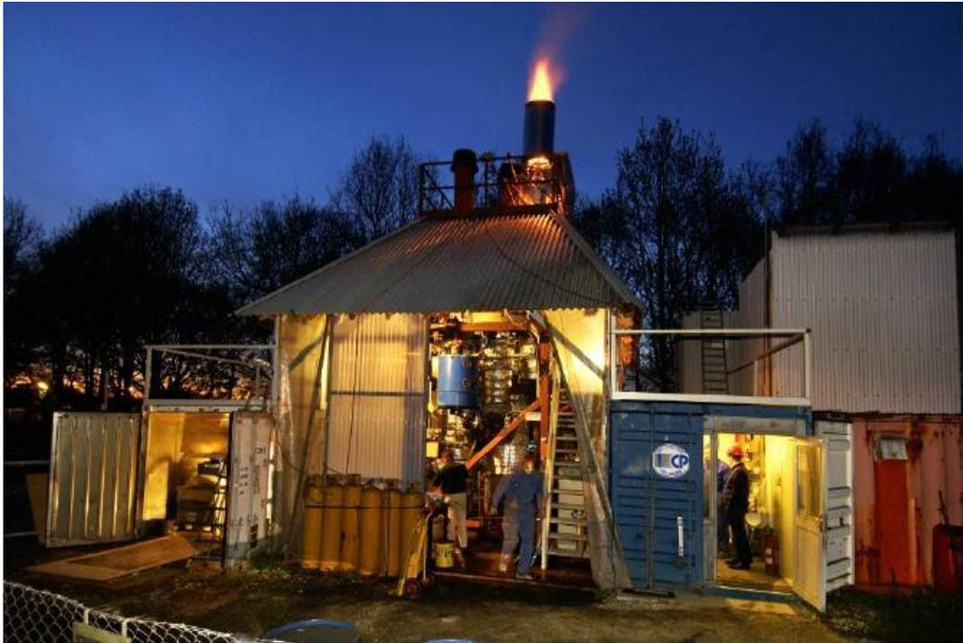
Figure 2.13 500 kW<sub>th</sub> LT-CFB test plant at DTU
