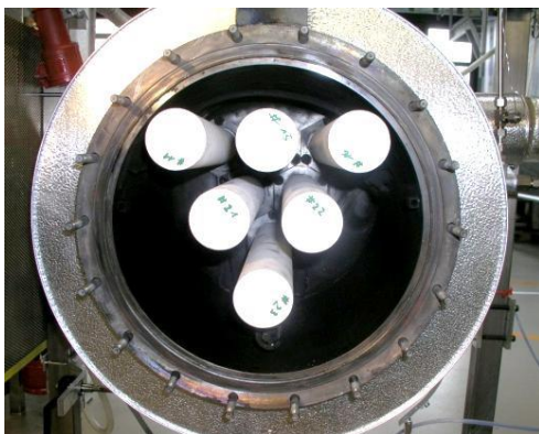
Figure 3.3: Filter elements with closed filter end acting as safety filter
