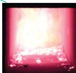
Left: Wood burns in the firebrick-lined firebox. Note the wood is only burning on the bottom due to downdraft design.
