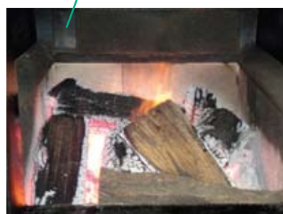
Left: Wood burns in the firebrick-lined firebox. Note the wood is only burning on the bottom due to downdraft design.
