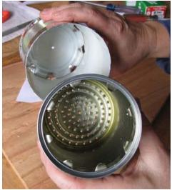
**Step 5: Assemble the inner and outer cans**
