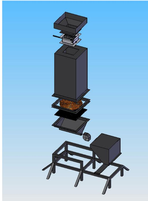
Figure 3. Downdraft gasifier (Capareda, 2006).
