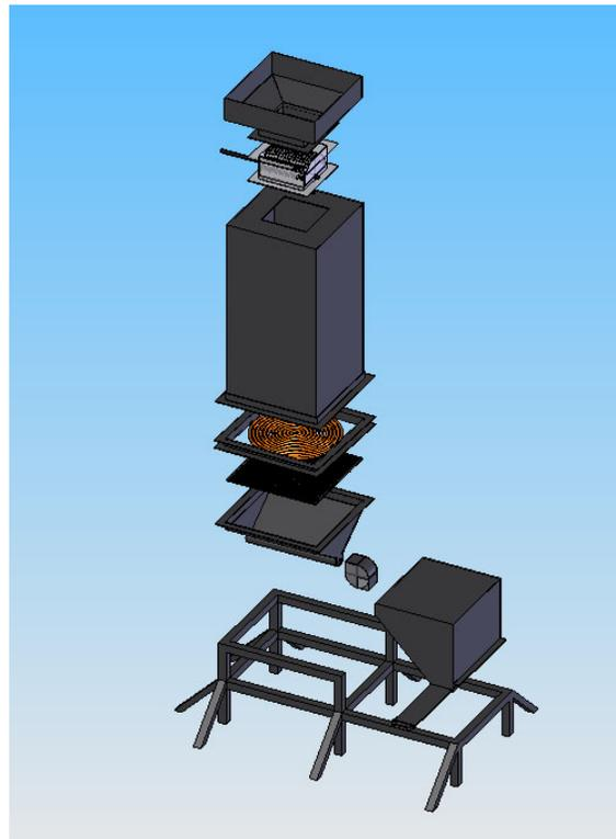
Figure 3. Downdraft gasifier (Capareda, 2006).
