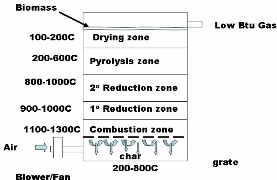
Figure 1. Schematic of an updraft gasifier (Capareda, 2006).
