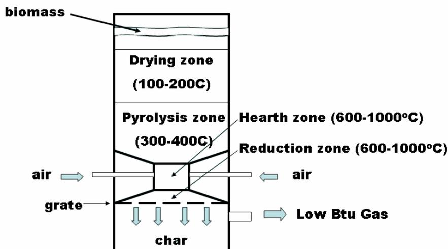
Figure 2. Schematic of a downdraft gasifier (Capareda, 2006).
